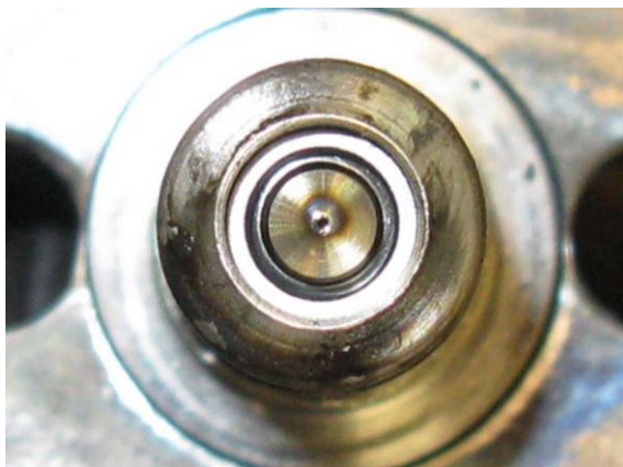
Figure 10: Close view of an injector nozzle from the 6 o'clock position with no blockages evident
