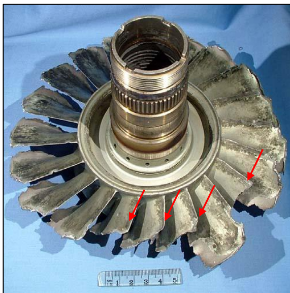
Figure 3: Typical failure blade cross-section
