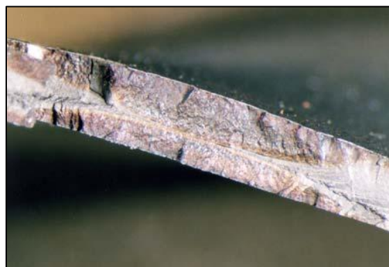
Figure 5: Failed blade cross-section – VH-EKX
