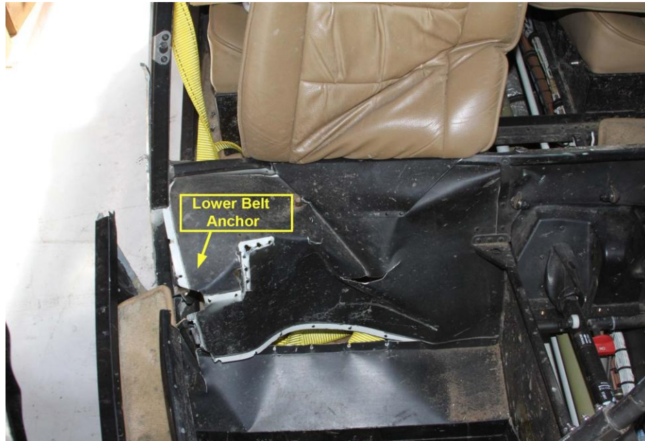
Figure 8: View of the pilot's seat showing where the lower belt anchor bracket had been attached to the seat/airframe structure
