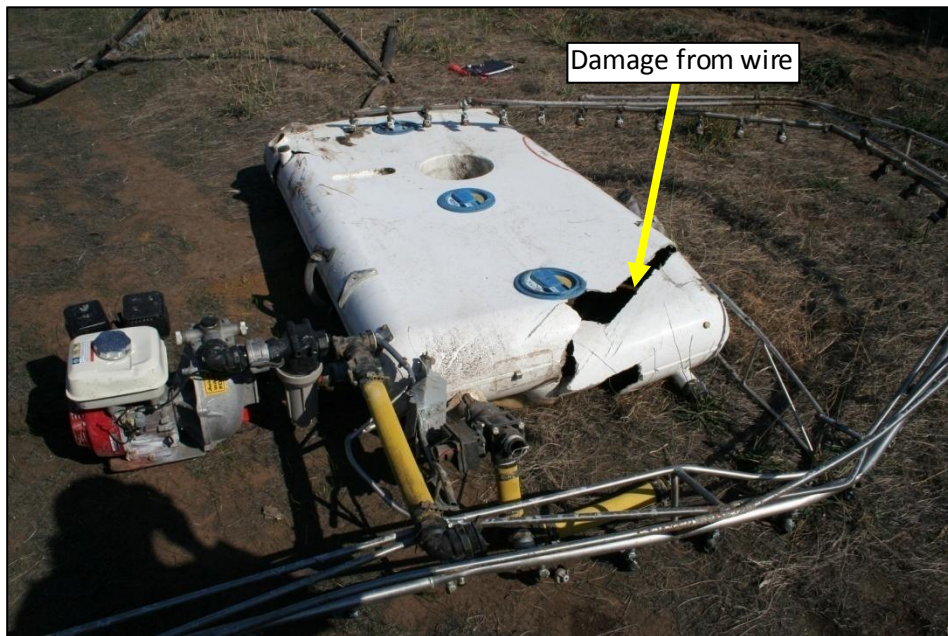
Figure 6: Overview of the reassembled spray tank showing the damage caused by the powerline
