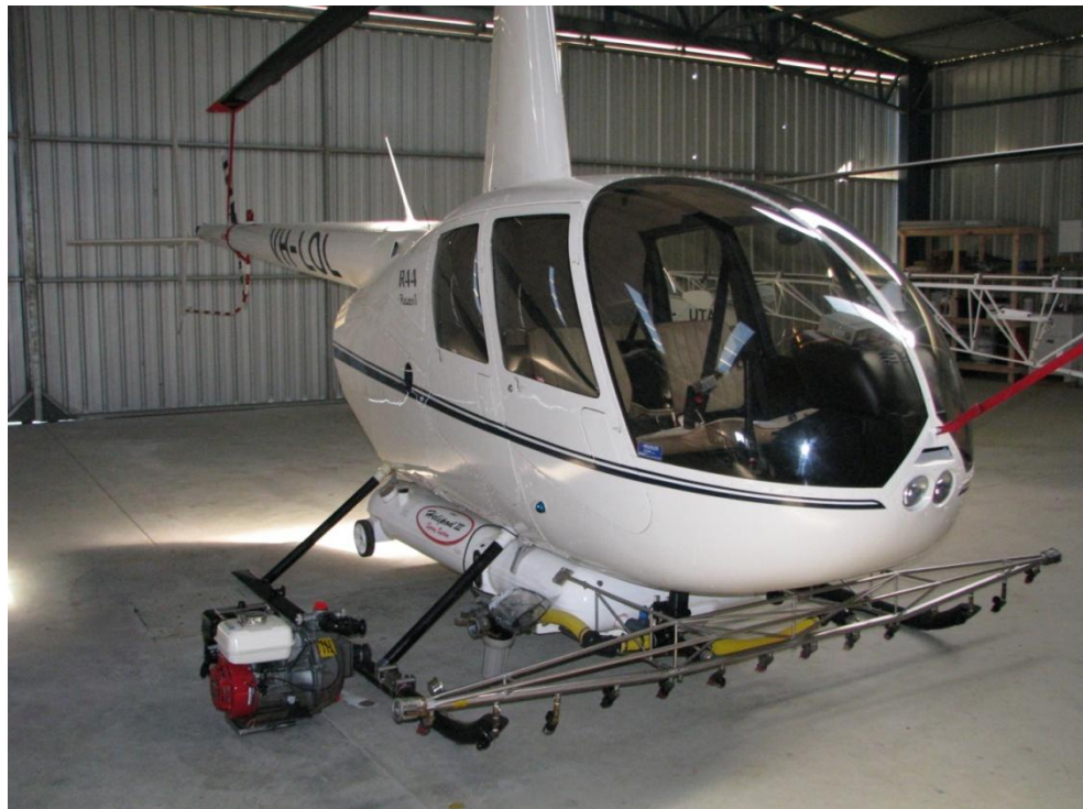
Figure 3: Operator's Helipod III spray system configuration
