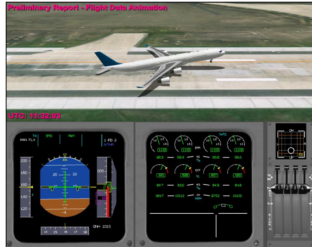
Figure B2: Initial tail contact with the runway
