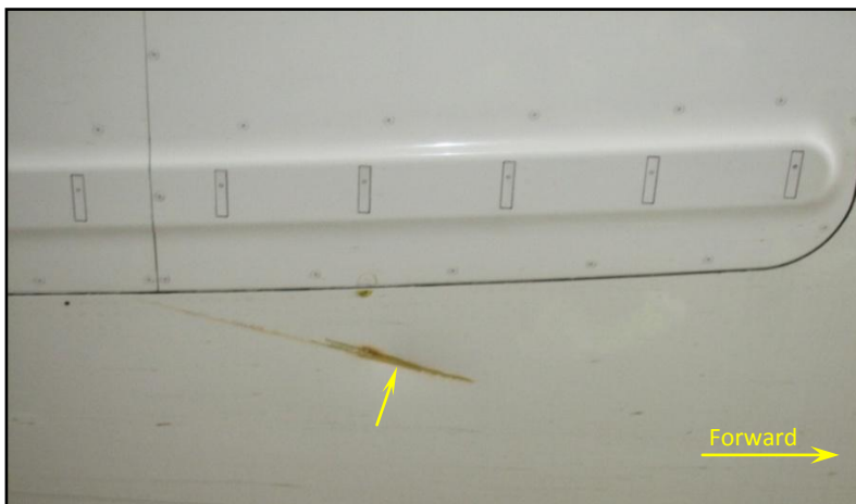
Figure 5: Contact mark below right, rear cargo door
