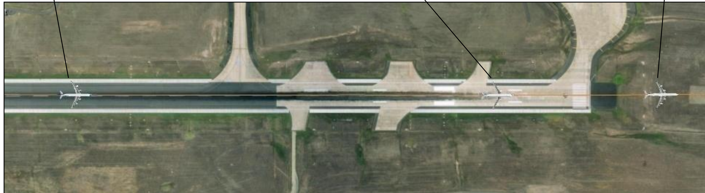
Figure B4: Graphical representation of the DAR data showing the position of the aircraft at a computed airspeed corresponding to V_1 as used by the crew, initial tail contact with ground, and final tail ground contact witness mark.
