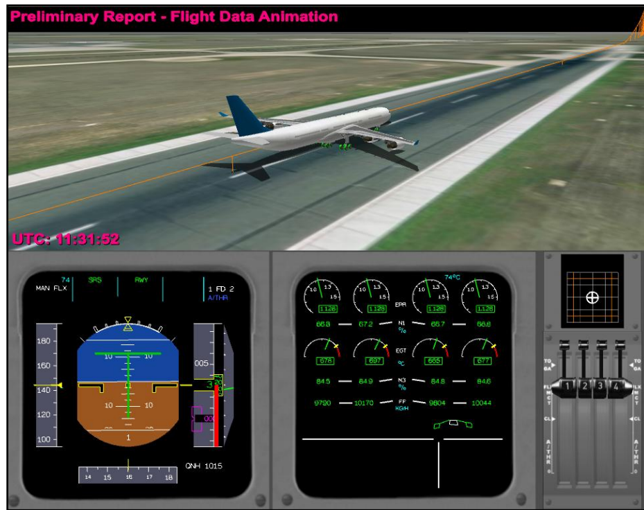
Figure B1: Aircraft attains computed airspeed of 143 kts corresponding to the V_1 used by the crew during the takeoff
