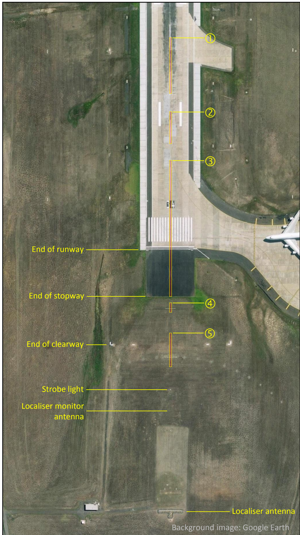
Figure 8: Ground contact marks
