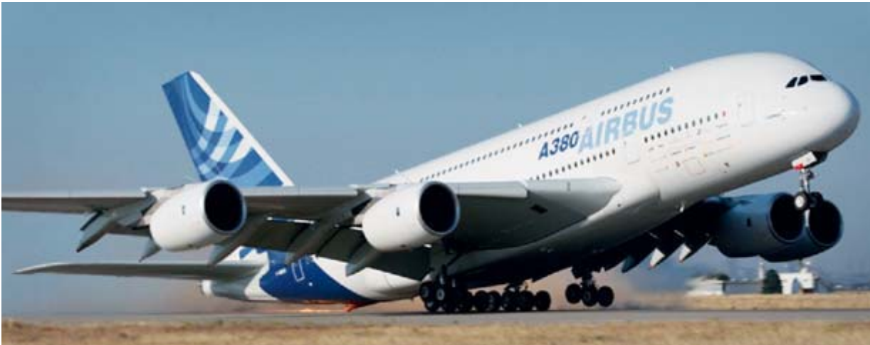
Figure 1: Minimum Unstick Speed (VMU) determination during flight test
