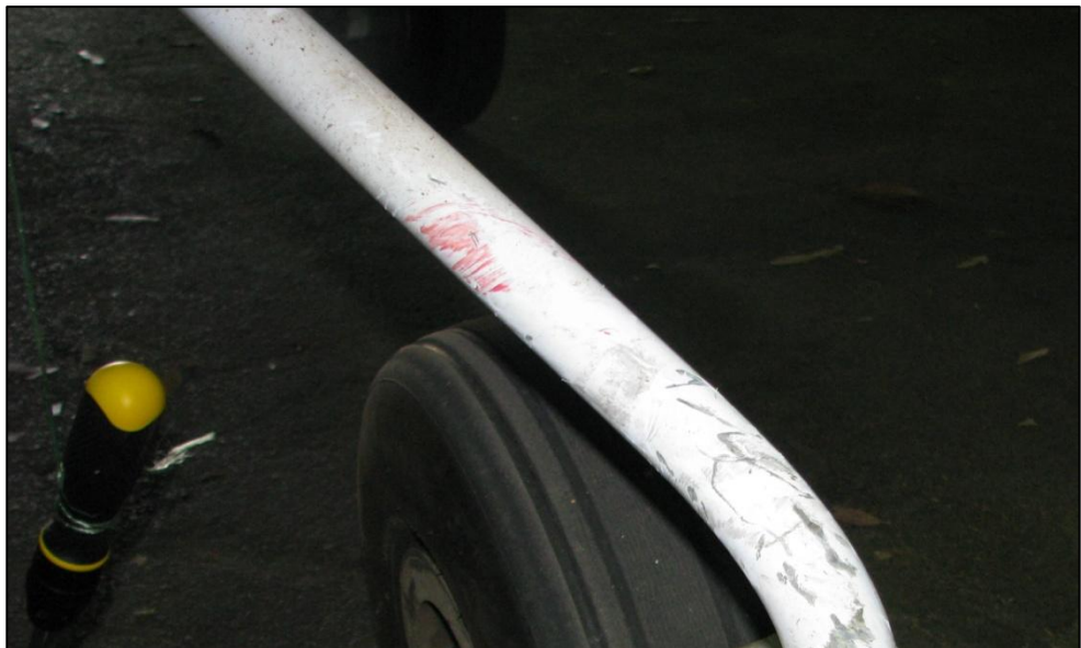
Figure 11: Red paint transfer on the right side of the nosewheel leg
