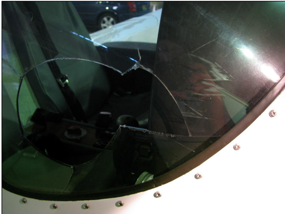
Figure 8: Broken right lower windscreen
