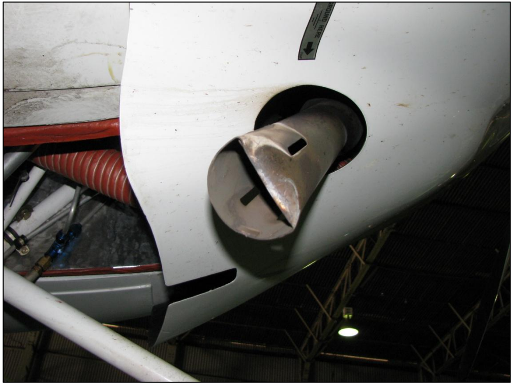
Figure 10: Exhaust pipe crush damage
