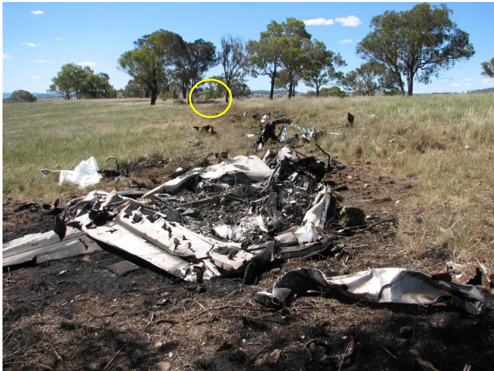
Figure 8: Main wreckage (looking back along the direction of approach – initial impact site circled)
