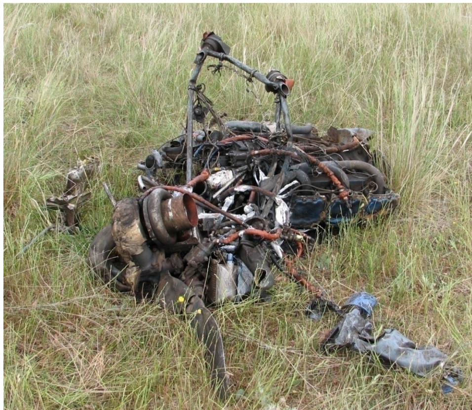
Figure 10: Left engine assembly as found on site
