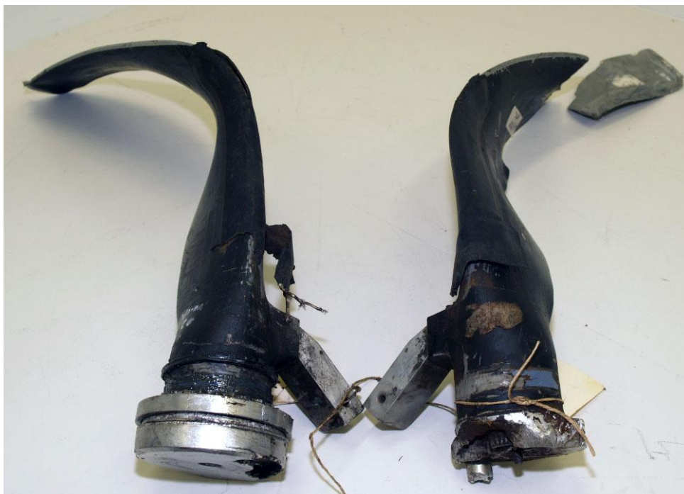
Figure 11: A left propeller blade (on left) and a right propeller blade (on right) with corresponding damage
