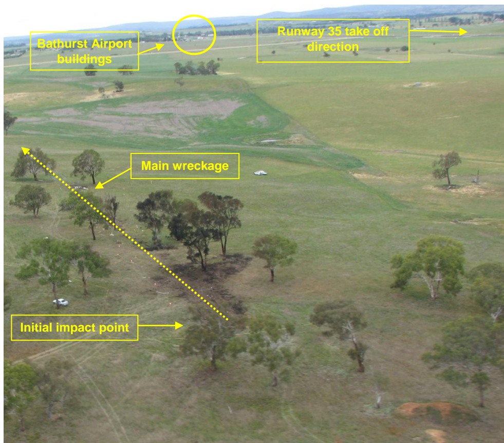
Figure 6: Accident site (dotted line indicates wreckage trail orientation)
