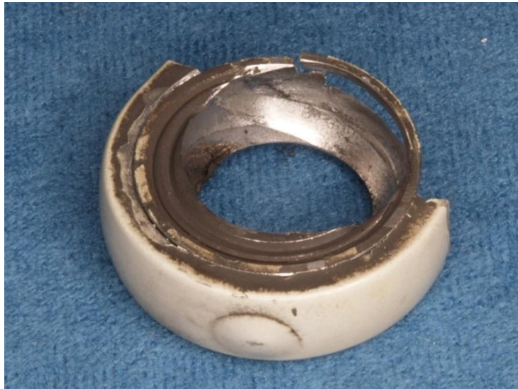
Figure 6b: Fractured rod end showing Teflon liner
