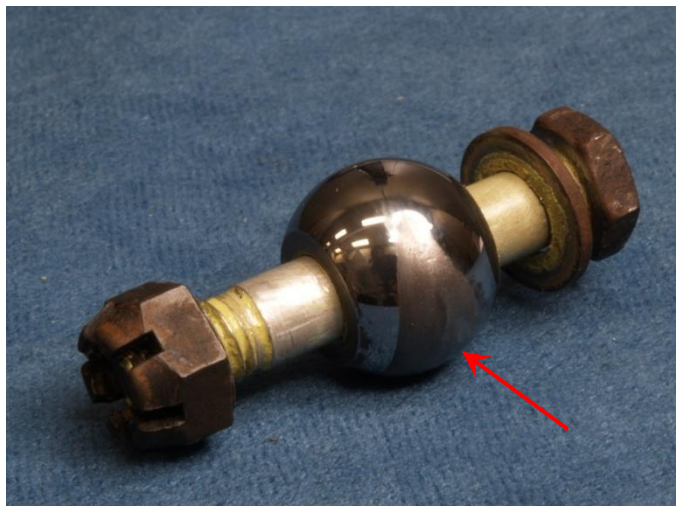
Figure 7: Ball wear, fractured pitch link
