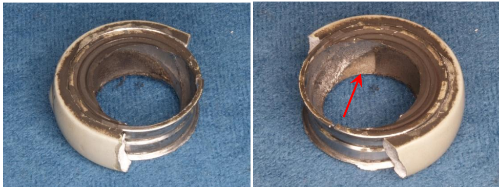
Figure 7: Ball wear, fractured pitch link
