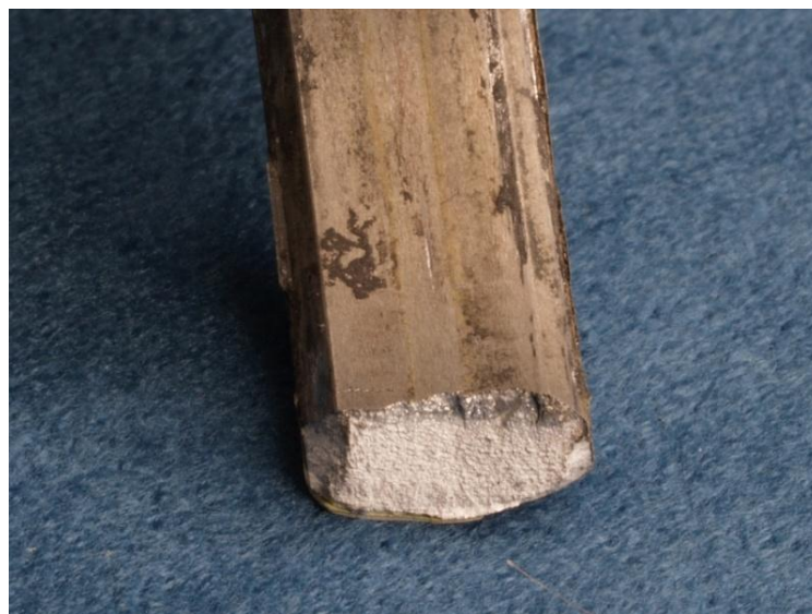
Figure 4b: Fracture surface at 10 o'clock position
