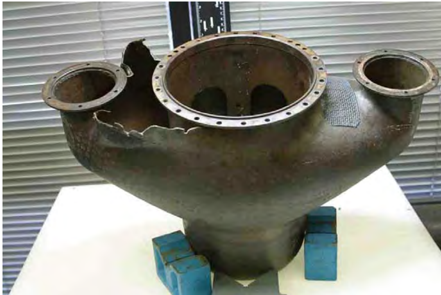
Figure A7: The primary point of failure in the left-side 'armpit' region
