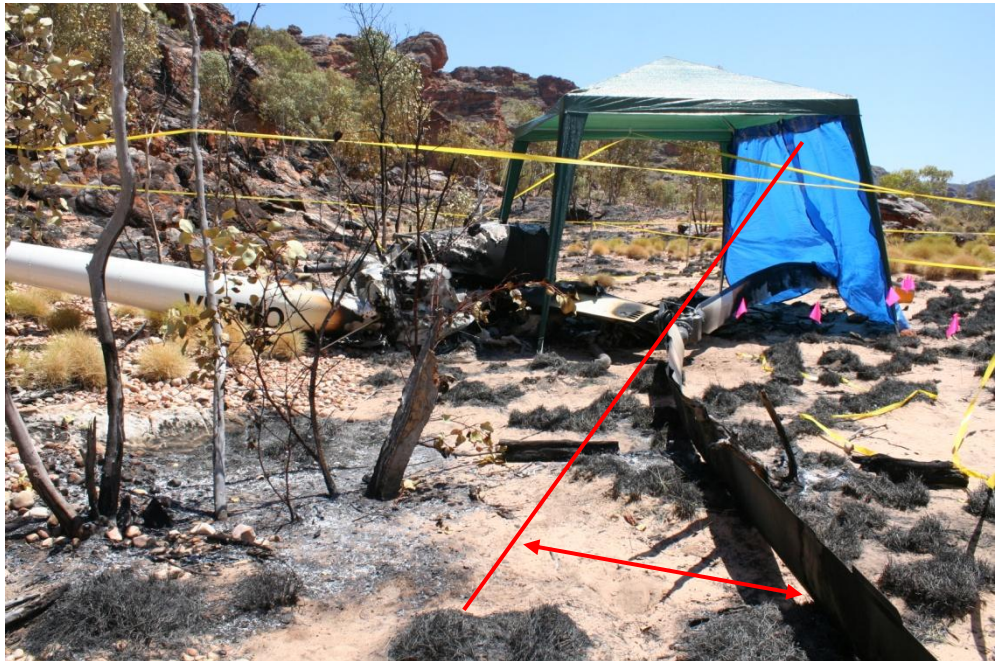
Figure 7: Main rotor blade coning (reference lines in red added)
