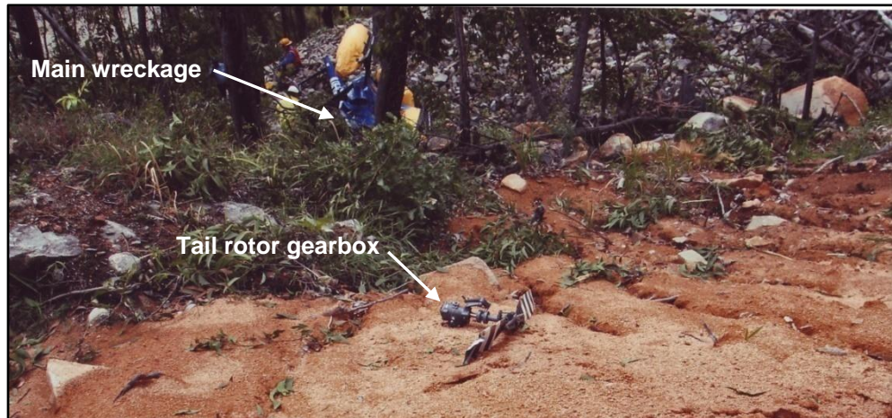
Figure 5: Detached tail rotor and gearbox
