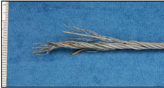
Figure 3: Cable fracture and associated strand separation
