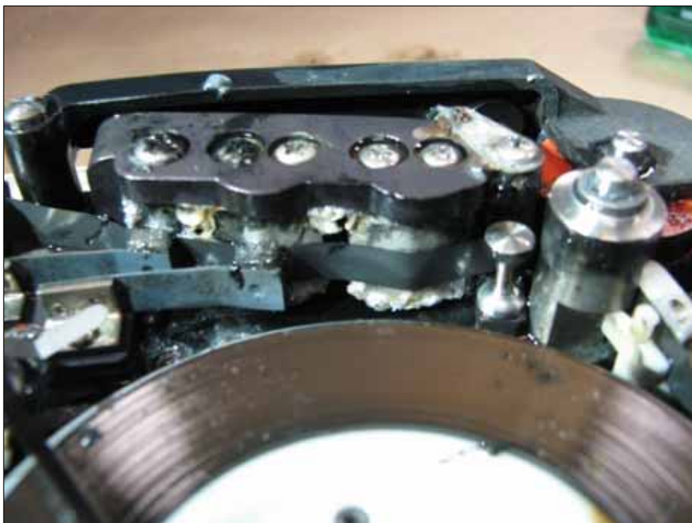
Figure B-27: CVR tape across erase and recording heads
