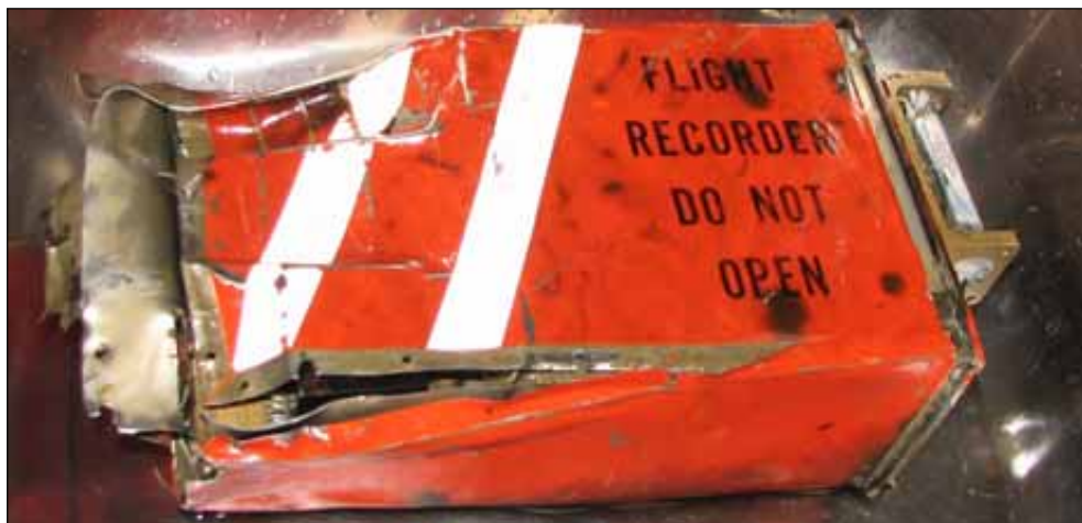
Figure B-21: Fairchild model A100A Cockpit Voice Recorder from VH-OZA following removal from shipping container on 1 July 2008
