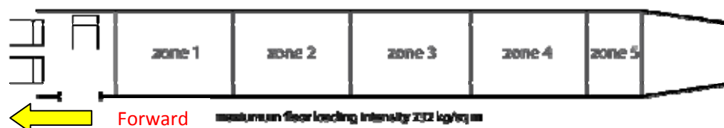
Figure 10: Metro III cabin loading layout
