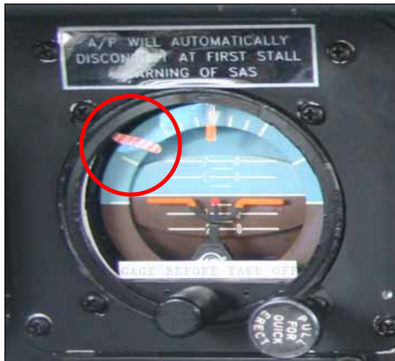
Figure 26: VH-OZN, pilot's AH with off flag visible (circled)
