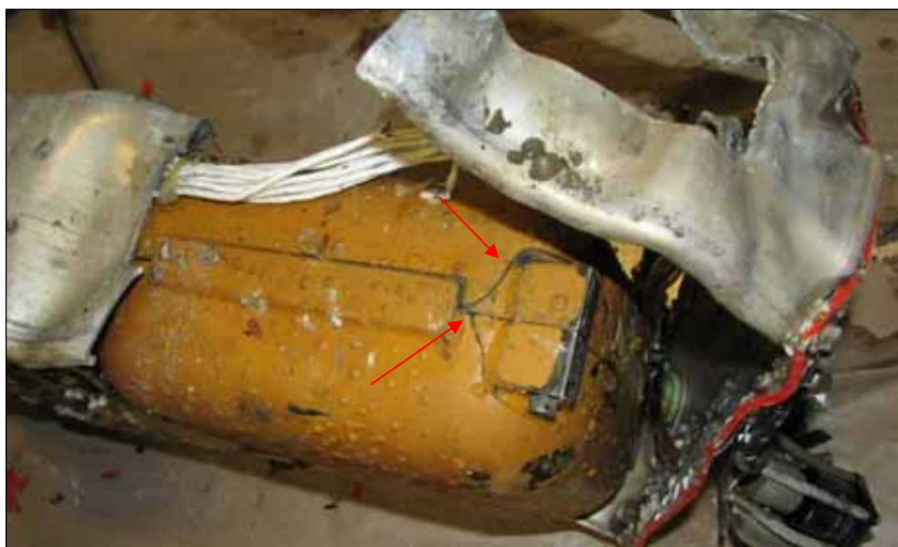
Figure B-7: FDR crash protected enclosure showing fracture damage (arrowed)
