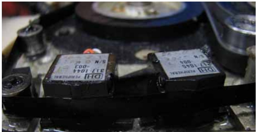
Figure B-11: Tape adhesion to tape transport heads
