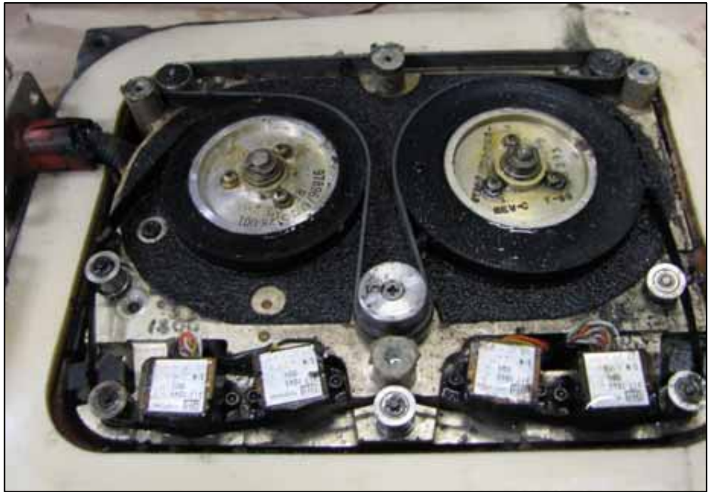
Figure B-11: Tape adhesion to tape transport heads
