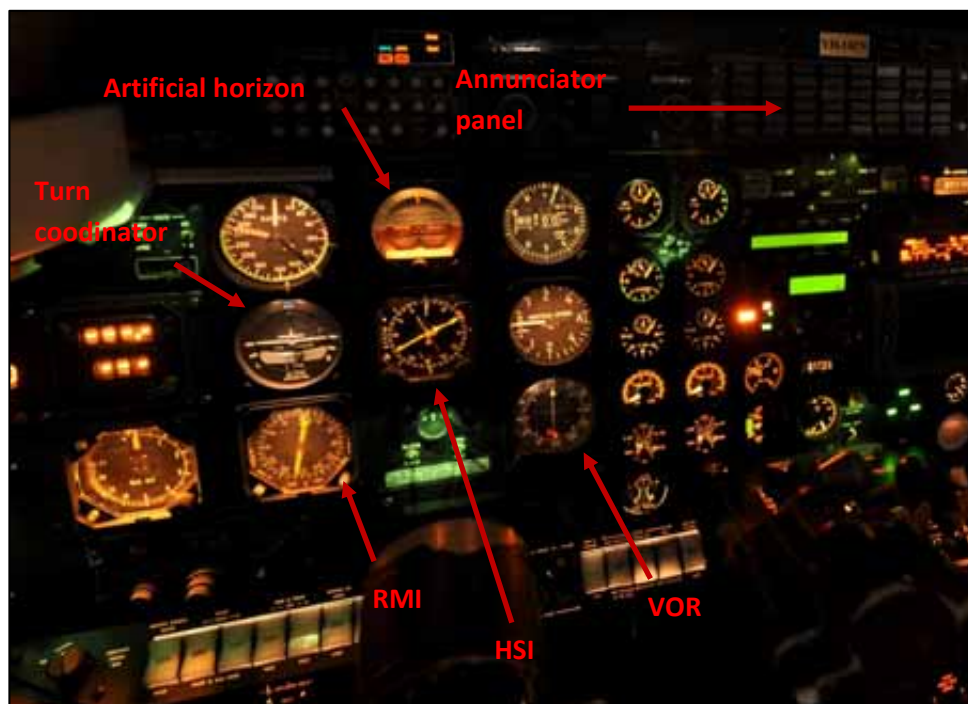
Figure 24: VH-OZN instrument panel during simulated normal night operations (pilot side) with no warning/caution lights or flags visible
