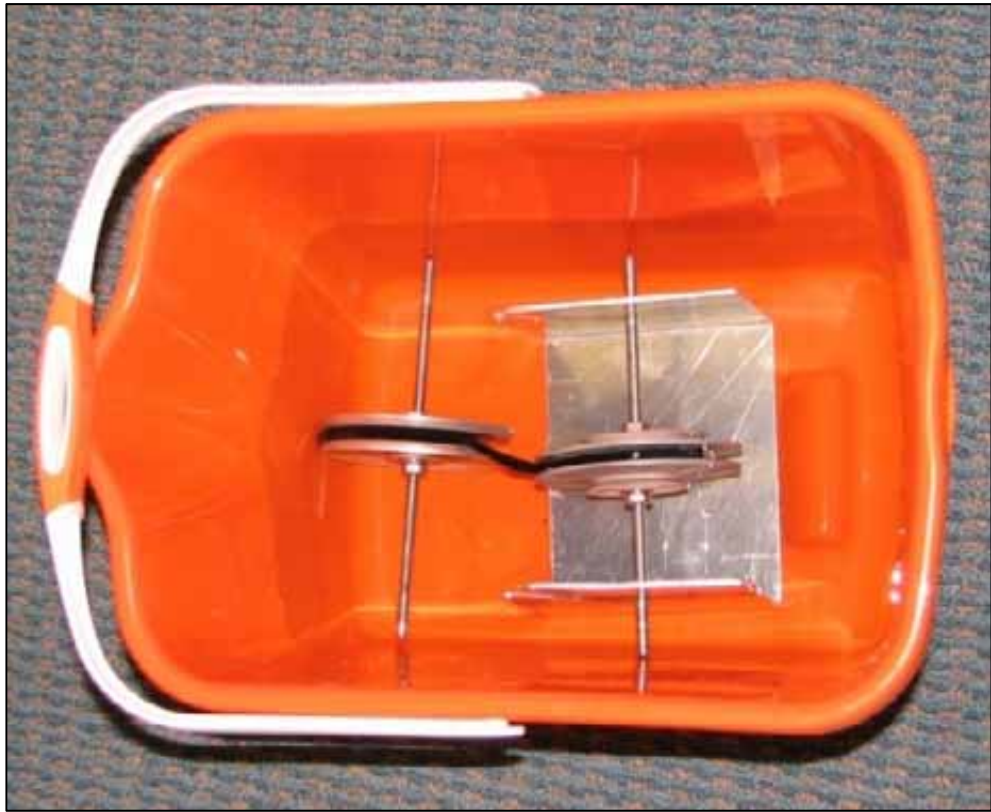
Figure B-12: Tape removed from FDR rinsed and cleaned and on spools
