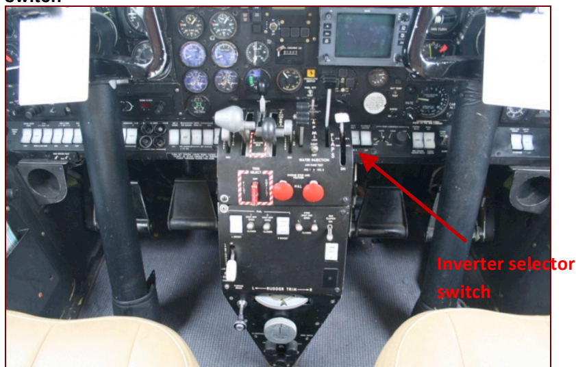
Figure 15: Cockpit layout of OZN, showing the location of the inverter selector switch
