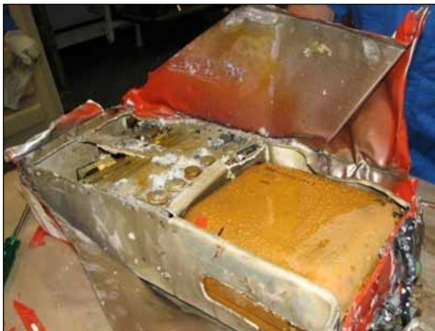
Figure B-7: FDR crash protected enclosure showing fracture damage (arrowed)
