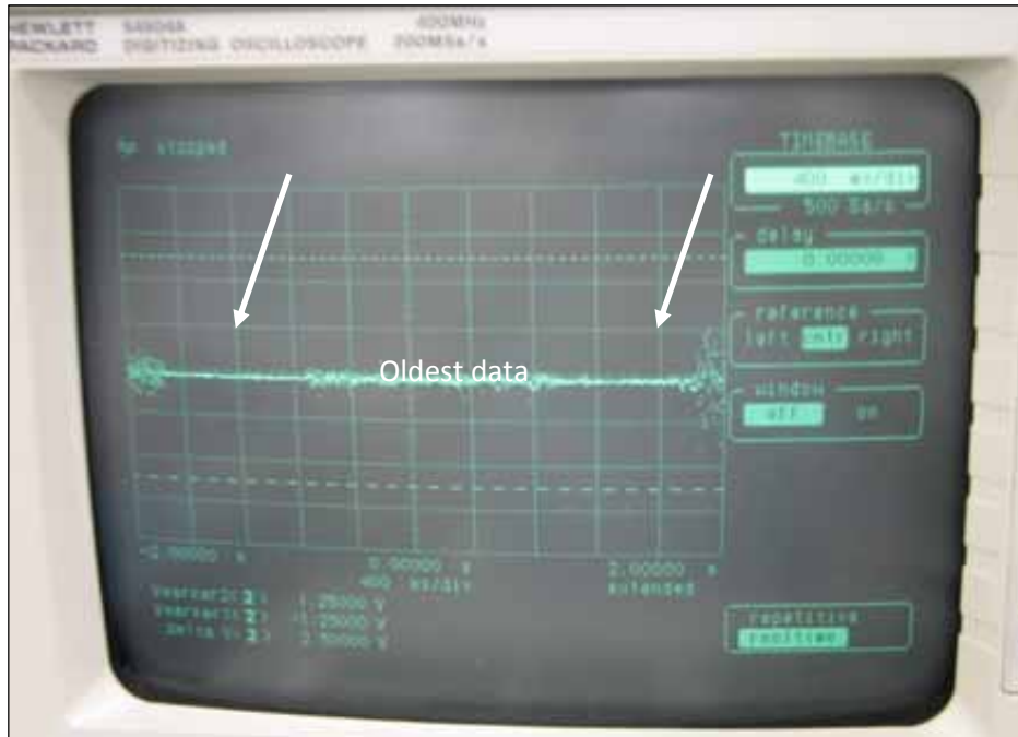
Figure B-14: Oscilloscope screenshot of Track 6 at location of tape stoppage (i.e. transition from newest to oldest data). Reduced signal strength arrowed. This was typical across all eight tracks
