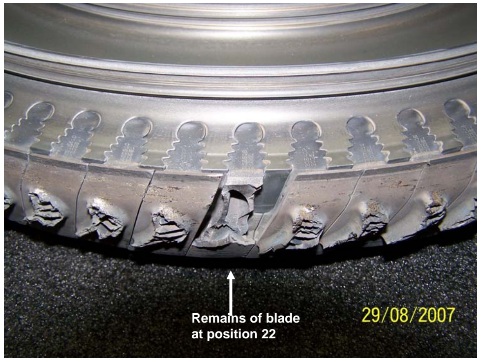
Figure 4: Damage to high pressure turbine stage 1 rotors
