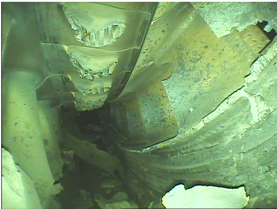
Figure 1: High pressure turbine stage-1 blade damage
