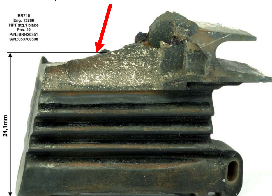
Figure 5: HPT stage 1 blade, position 22 showing overview of the blade pressure side where the crack initiation occurred
