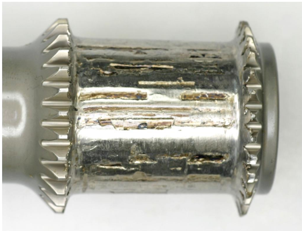
Figure 12: Photograph of the sun gear showing complete 'machining' wear of the teeth that had normally engaged with the planet gears
