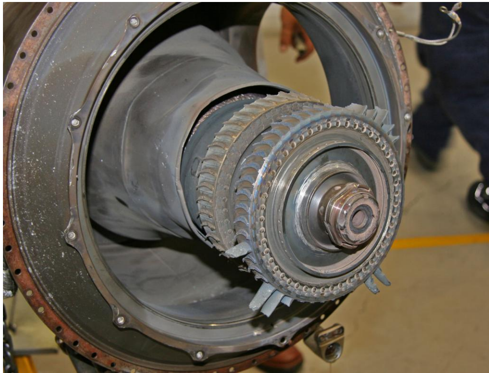
Figure 3: Close-up of the ruptured gas generator case showing the exit path of the fractured power turbine blades
