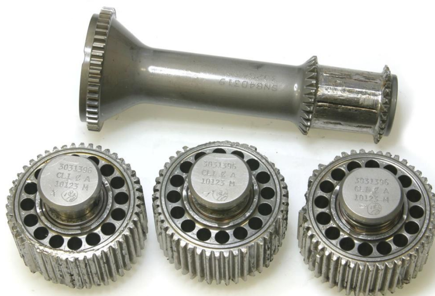
Figure 8: The sun gear and planet gear set from the first-stage reduction gear assembly
