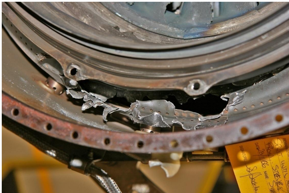
Figure 3: Close-up of the ruptured gas generator case showing the exit path of the fractured power turbine blades
