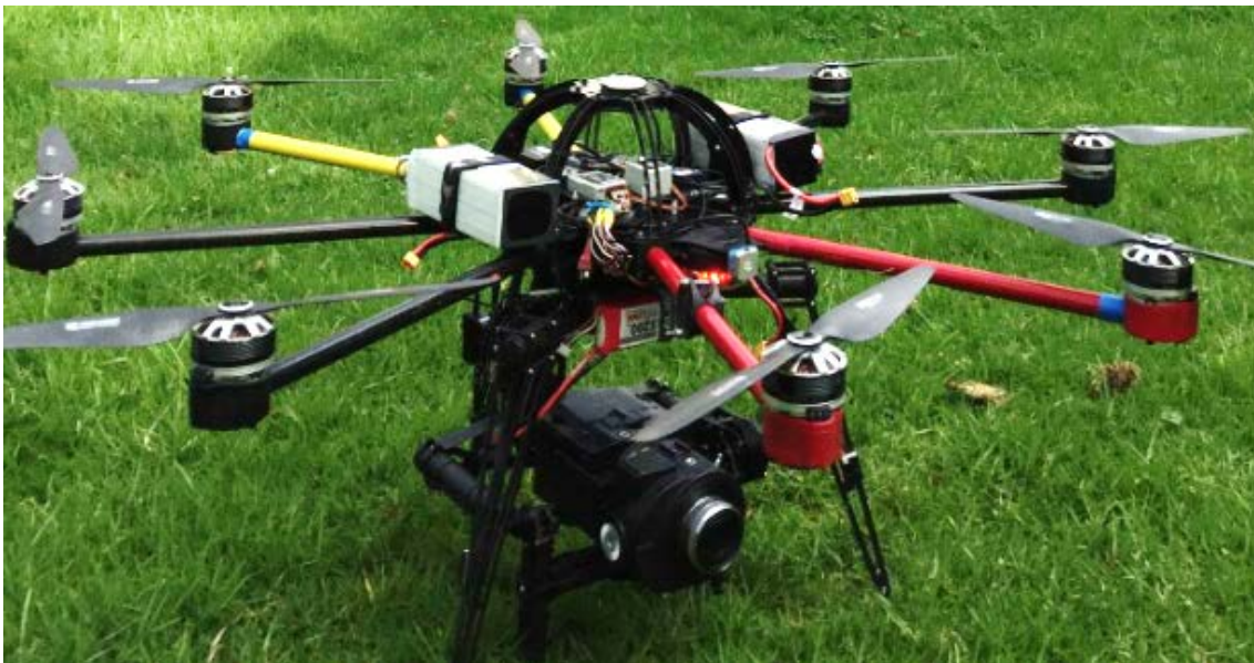
Figure 1: RPA prepared for flight with camera mounted beneath
