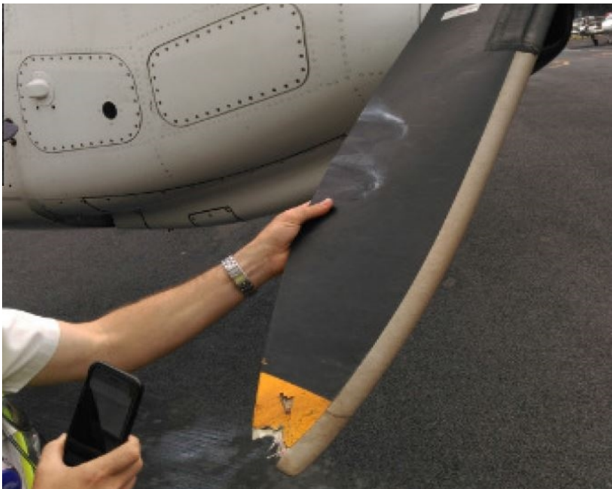
Figure 2: Left engine propeller showing damaged blade tip on arrival at Merimbula
