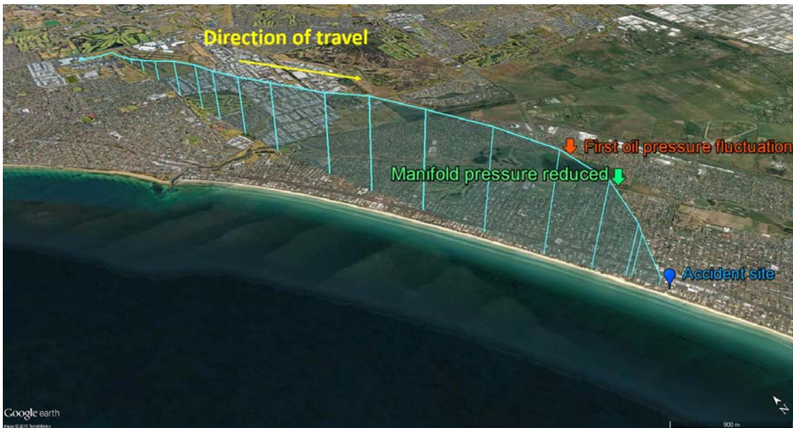
Figure 5: Downloaded GPS track, and the position of the first oil pressure fluctuation and reduction in engine manifold pressure
