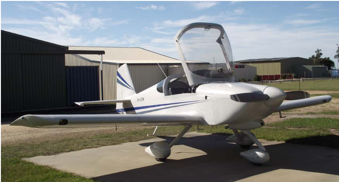
Figure 2: JON showing the tip-up canopy in the open position
