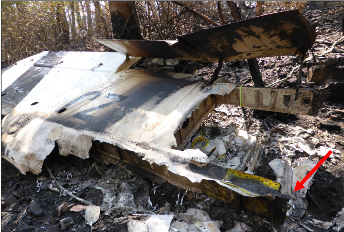
Figure 6: Outboard left wing (underside of wing visible, lower attach fitting arrowed)
