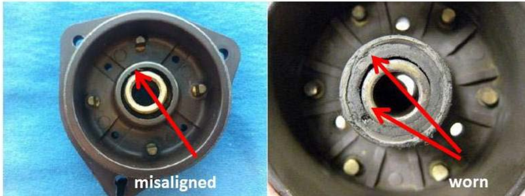
Figure 2: Two examples of unserviceable distributor blocks
