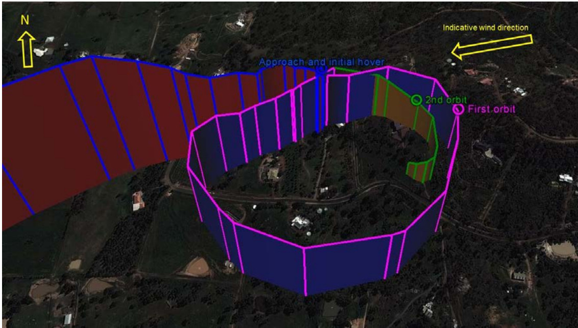
Figure 7: GPS data representing the helicopter's track and height in vicinity of the accident site
