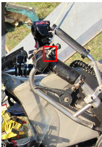
Figure 9: Hydraulic cut-off switch – VH-RDU (left) and a typical installation (right)
