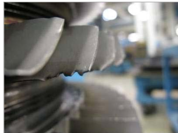
Figure 4: Example of HPC rotor blade damage.
