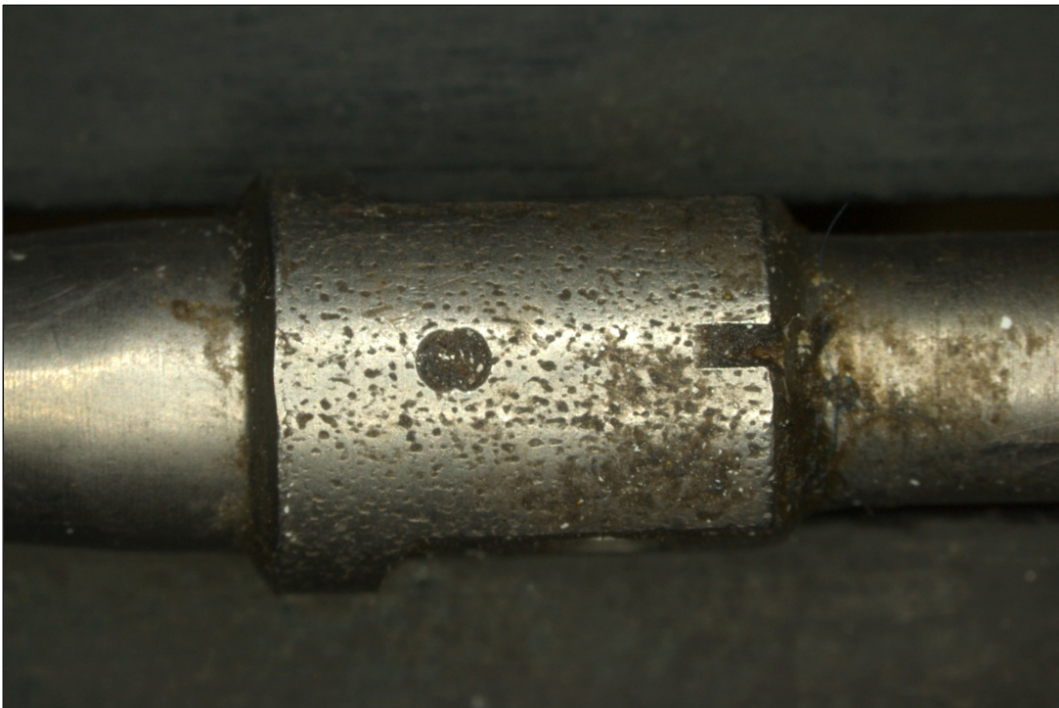
Figure 4: 'OO' terminal with discolouration and rough/pitted surface on the centre section.
