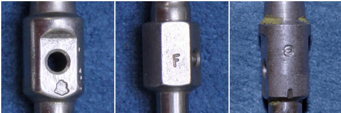
Figure 2: Manufacturer markings observed on the submitted terminals (from left to right; bell, F and OO)
