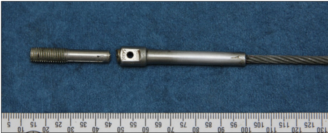
Figure 11: Failed terminal submitted to the ATSB
