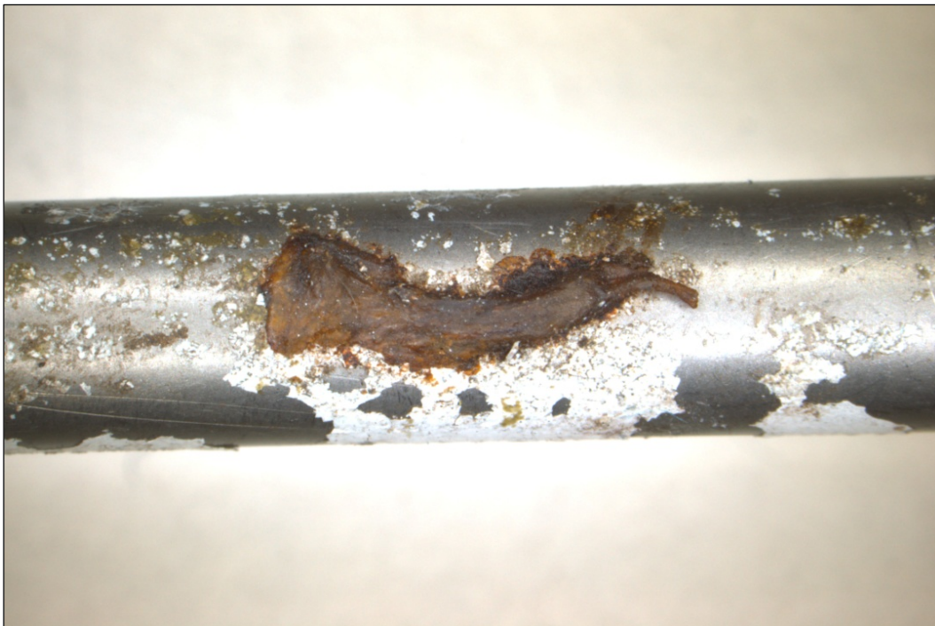
Figure 5: Deposit on the surface of sample 4; a 'bell' MS21260 terminal
