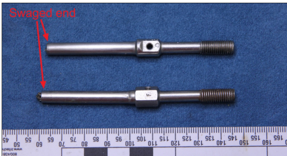
Figure 1: Sample of cable terminals submitted to the ATSB
