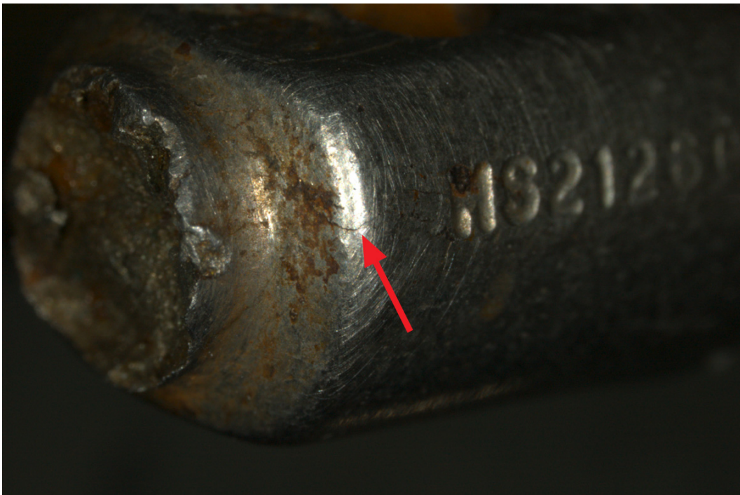
Figure 12: Widespread discolouration and secondary cracking (arrowed) on failed terminal
