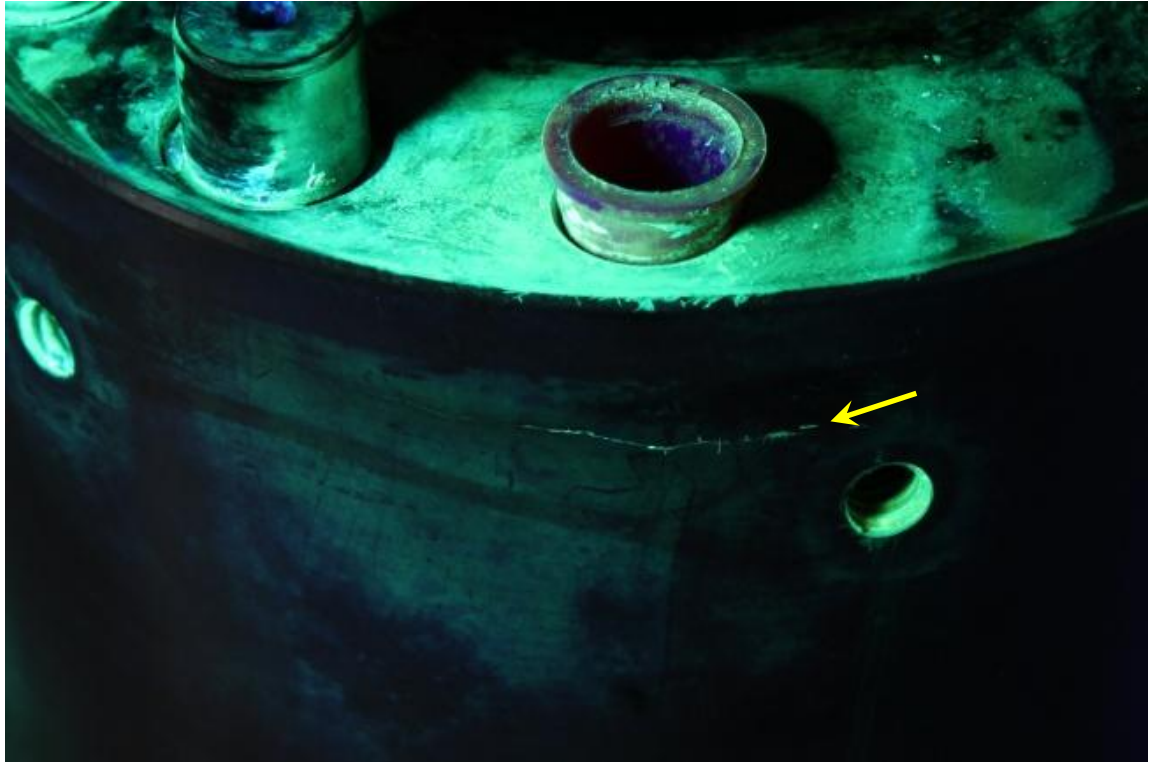
Figure 2: Fluorescent penetrant inspection with crack indications on the hub exterior (top) and interior (bottom)
