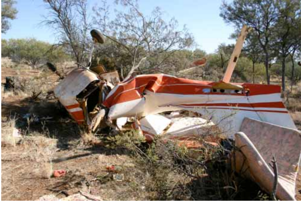
Figure 1. Right wing, horizontal stabiliser and main landing gear torn away, fuselage breached at the rear of cabin.
