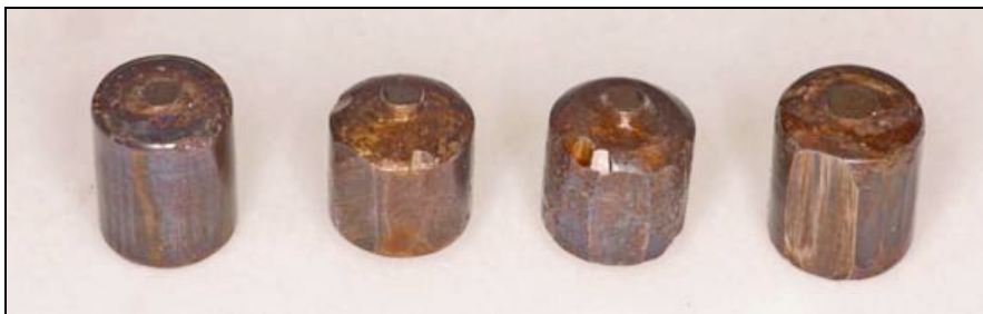
Figure 5: Selection of bearing rollers showing damage sustained
