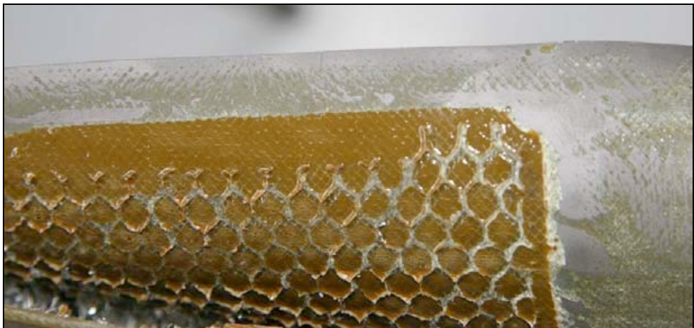
Figure 11: Disbonded skin surface, showing patchy adhesive and cohesive failure modes
