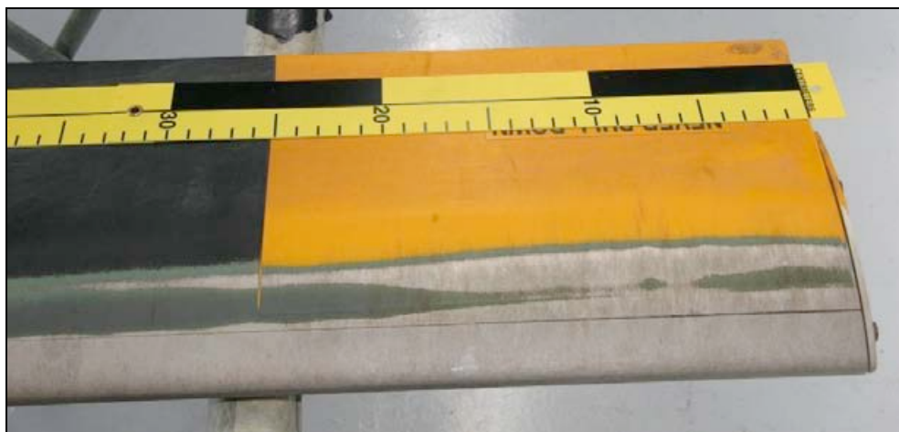
Figure 6: Erosion on the opposite blade (3519E) lower surface
