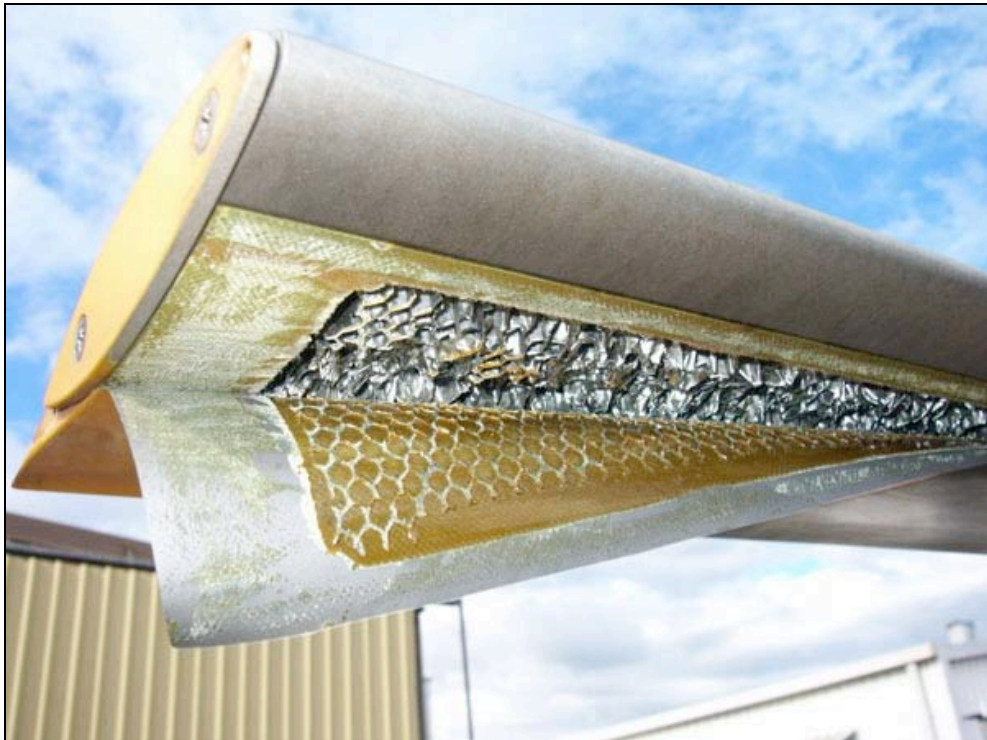
Figure 1: Separation of the main rotor blade lower skin, VH-HPI
