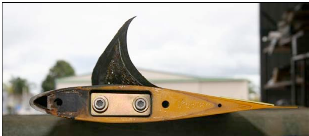
Figure 4: Extent of lifted skin projection from the aerofoil profile (blade upside-down)
