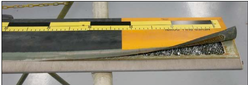
Figure 4: Extent of lifted skin projection from the aerofoil profile (blade upside-down)
