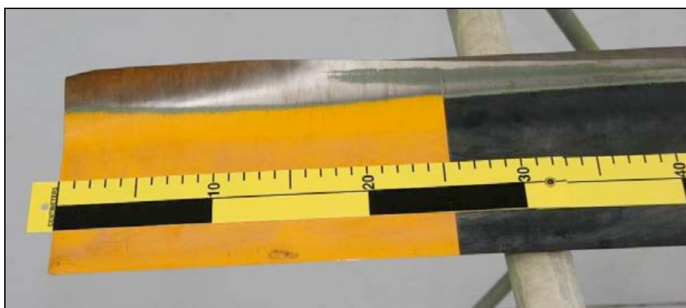
Figure 6: Erosion on the opposite blade (3519E) lower surface
