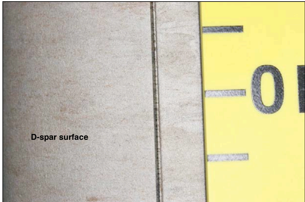
Figure 15: Closer view of voids and eroded areas along the bond line, blade 3519E. Larger void arrowed
