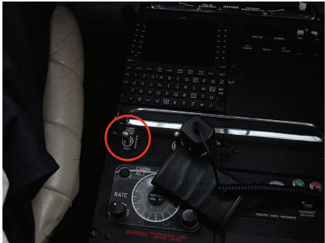
Figure 1: Pressurisation, dump and test switch location
