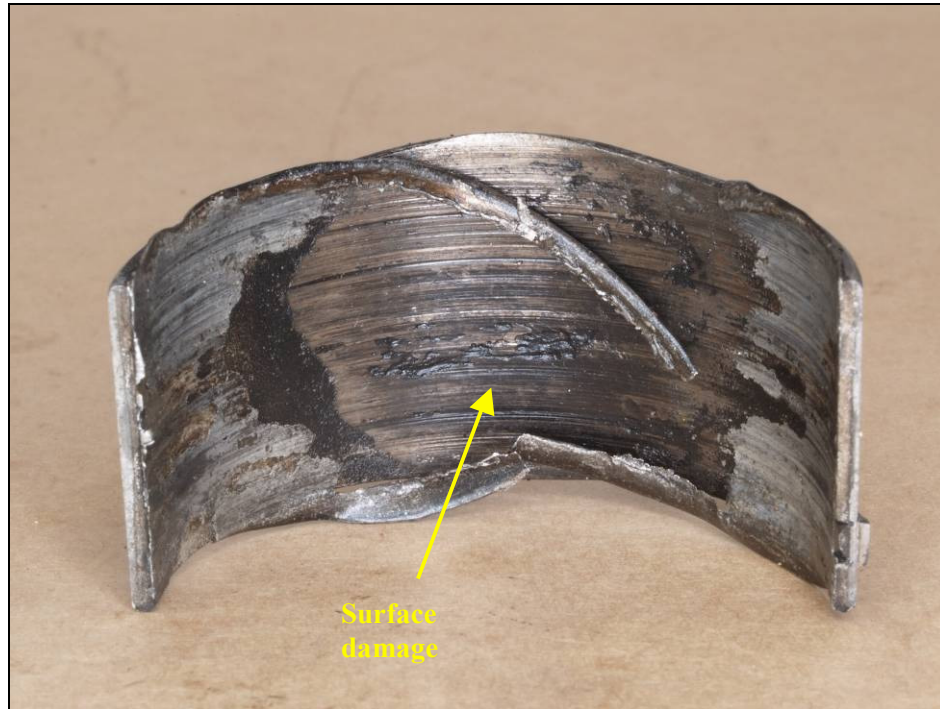
Figure 7: Right engine number-4 connecting rod crankshaft bearing (upper)
