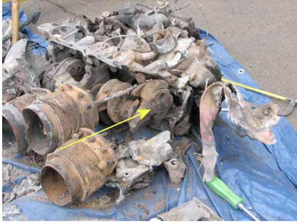
Figure 8: The right engine and fractured crankshaft (arrowed).
