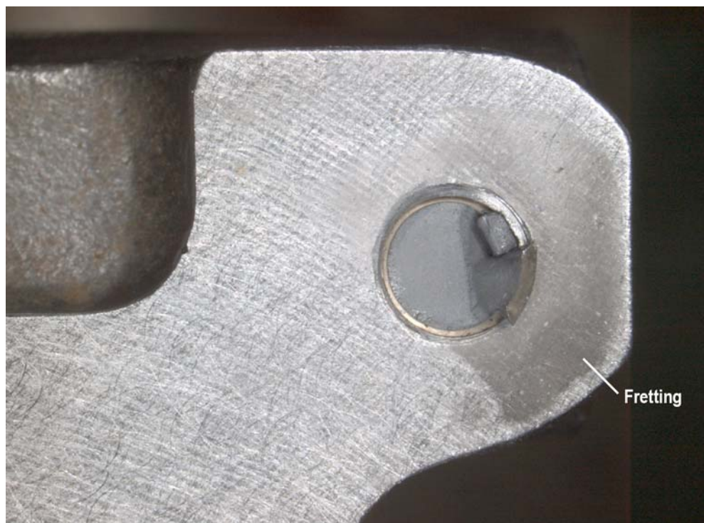
Figure 5: Fretting damage was found on the sequence valve flange surface, close to each of the broken fastener locations.
