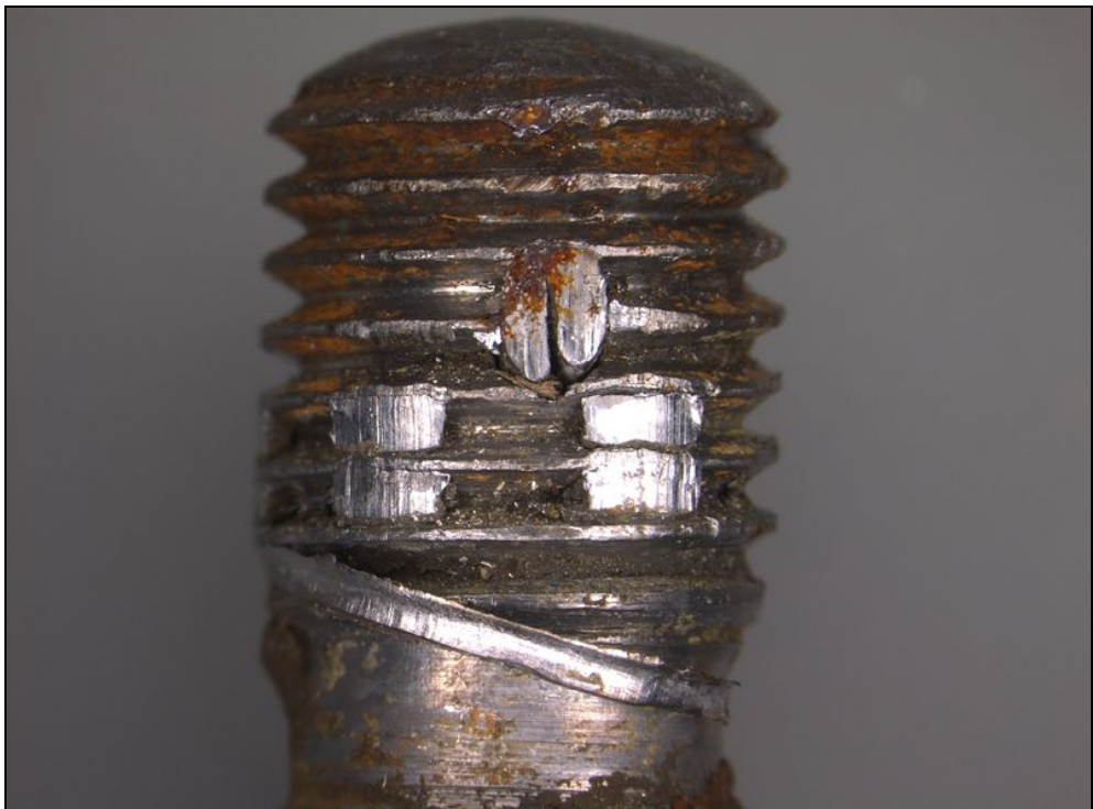
Figure 10: Thread remnants on rudder lower hinge pin
