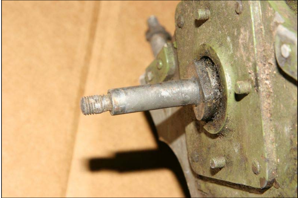
Figure 10: Thread remnants on rudder lower hinge pin
