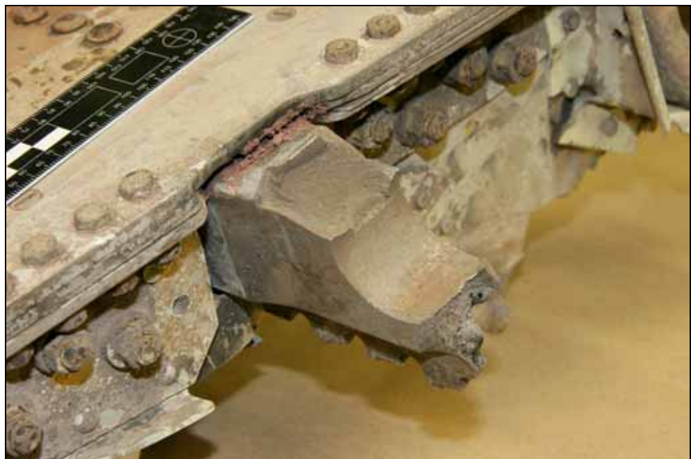
Figure 7. Fractured right wing upper attachment lug
