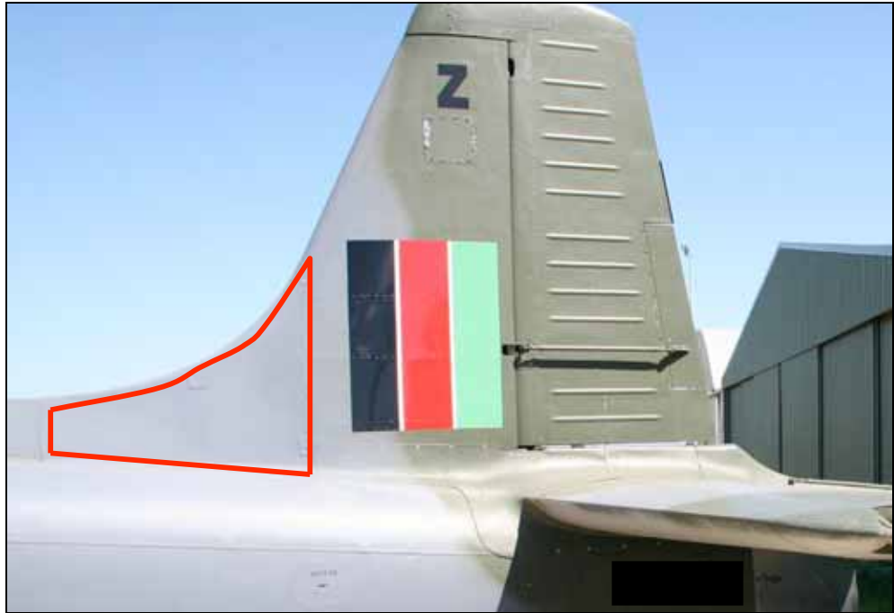
Figure 28: Location of fin-to-fuselage fairing (outlined)
