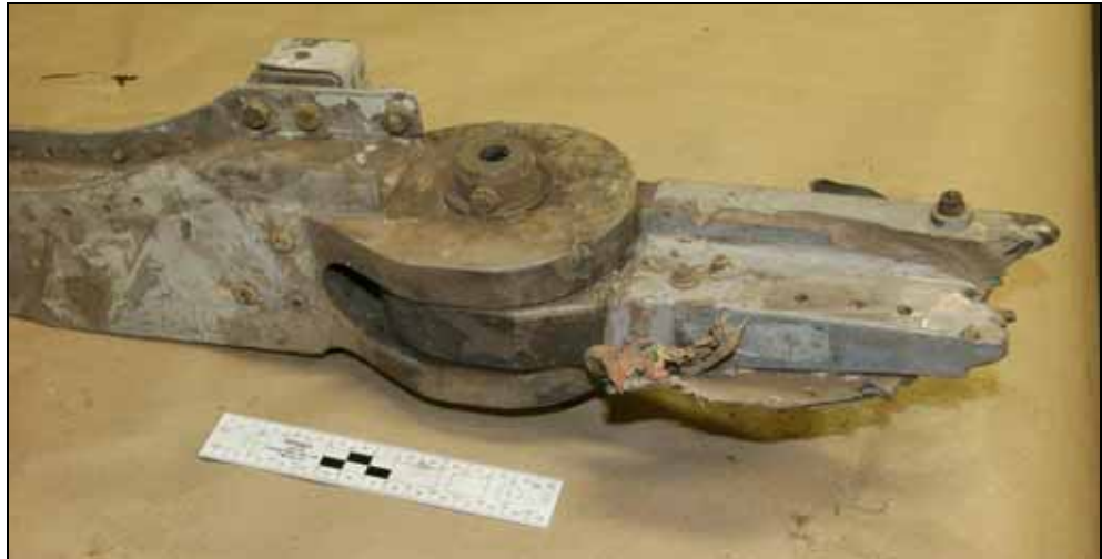
Figure 16. Fractured flange section outboard of the spar lower lug
