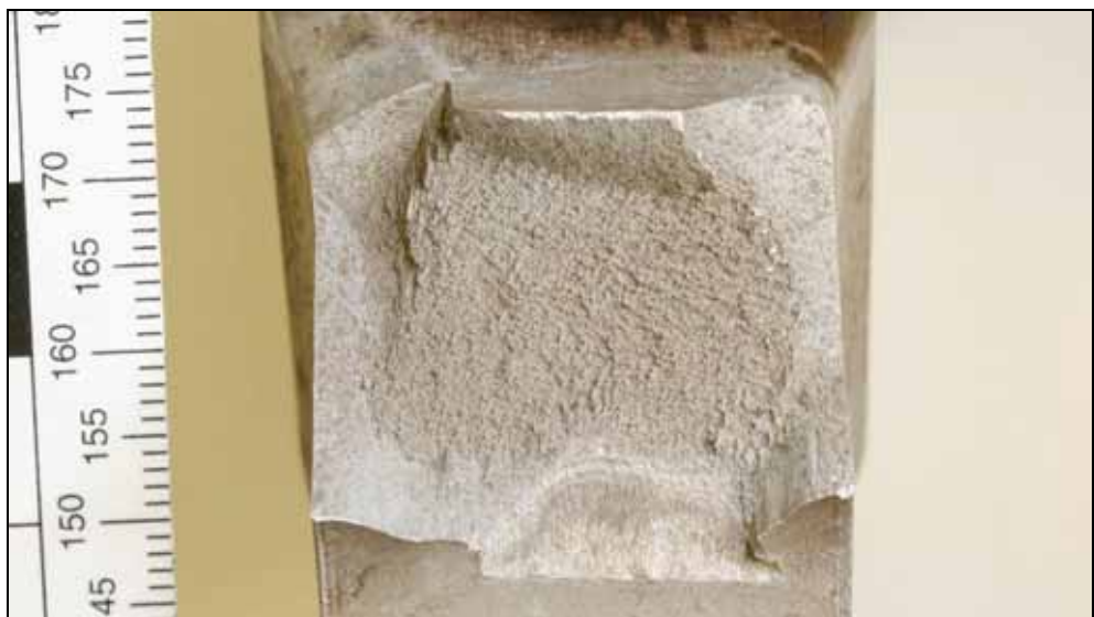
Figure 9. Fracture detail – right wing upper attachment lug
