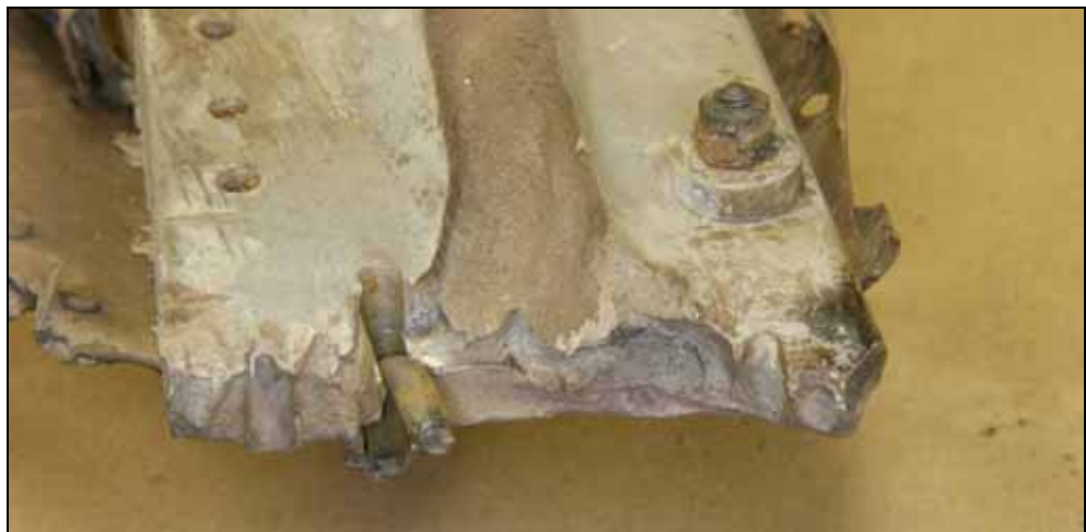
Figure 16. Fractured flange section outboard of the spar lower lug
