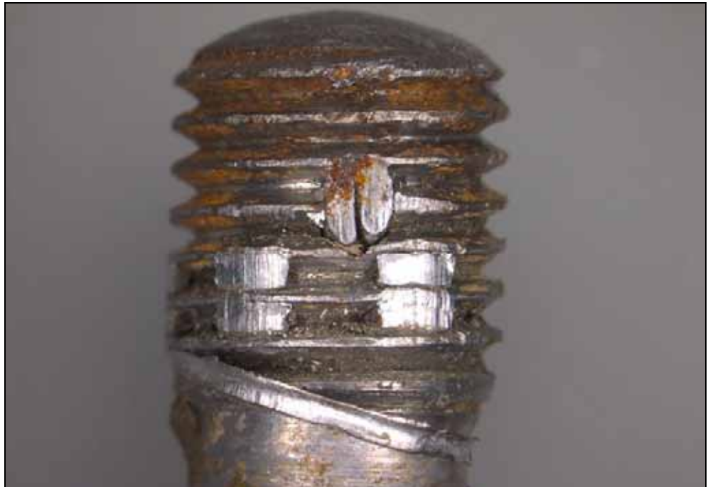
Figure 25: Thread remnants on rudder lower hinge pin
