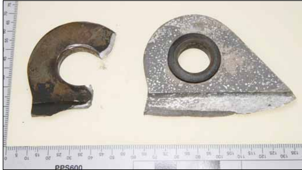
Figure 17. Right wing rear attachment yoke flanges
