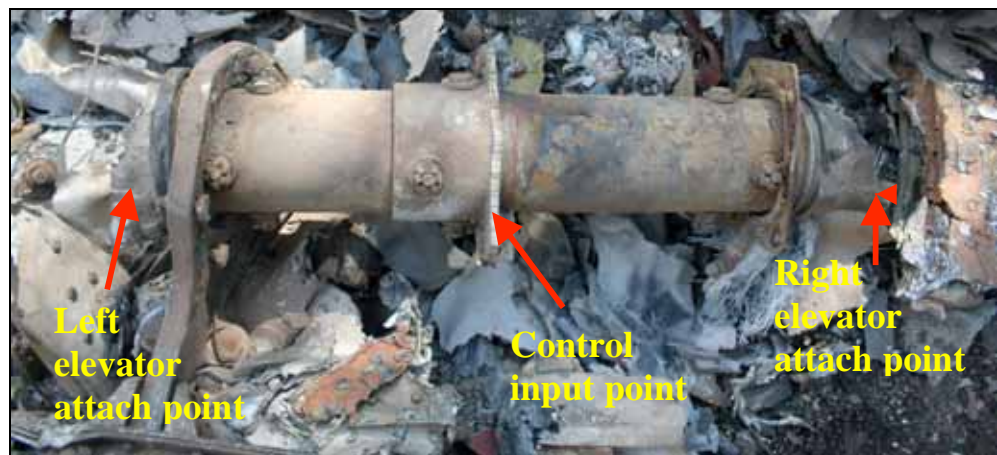
Figure 36: Elevator torque tube as found
