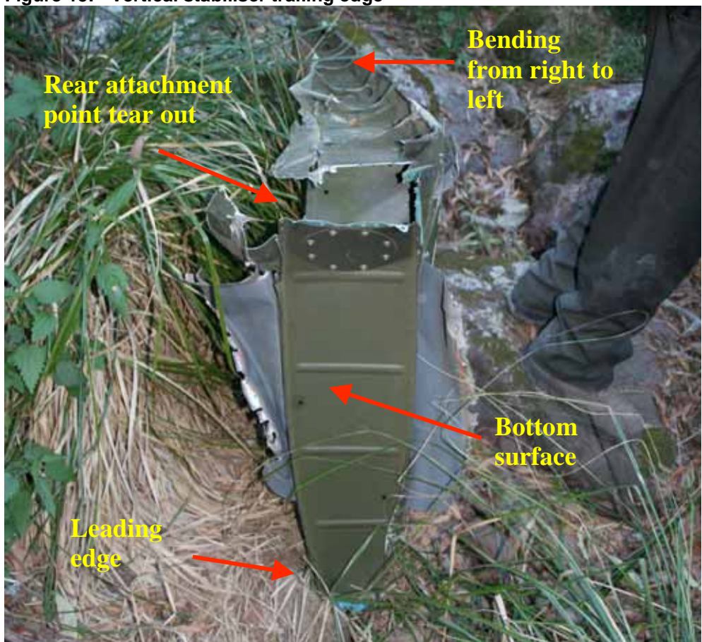
Figure 15: Vertical stabiliser trailing edge
