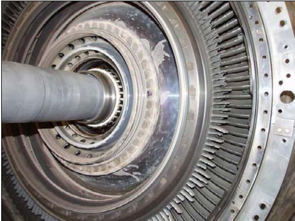
Figure 3: Damaged stage-1 LPT blades. View looking towards the rear of the engine
