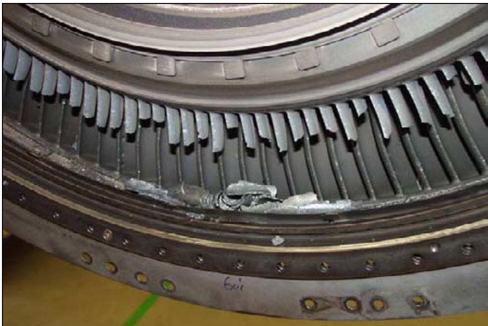
Figure 4: Stage-1 LPT disk and blades, with accumulated blade debris
