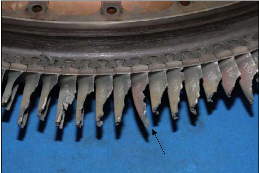
Figure 5: Damaged LPT stage-1 blades. Note the variation in colouration and curvature shown (example arrowed)
