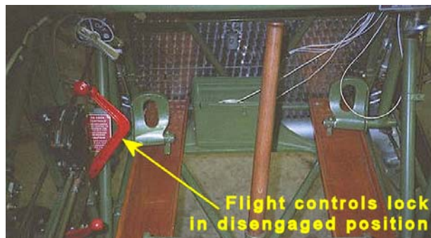
Figure 2: Flight controls lock on N73410 before the accident
