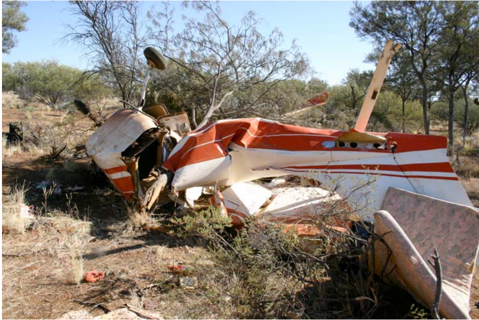
Figure 2. Fuselage breached at the rear of cabin with right wing, horizontal stabiliser and main landing gear torn away
