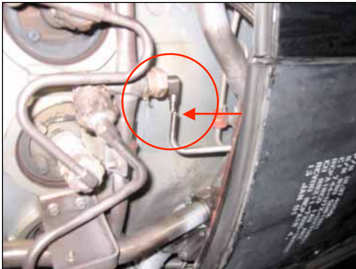
Figure 1: Previous fuel manifold drain line fracture
