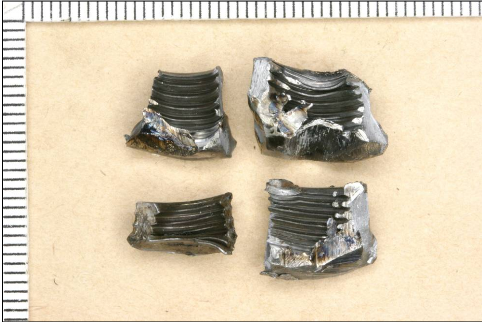
Figure 8: Fragments of nut from number-5 connecting rod bolt 'B'
