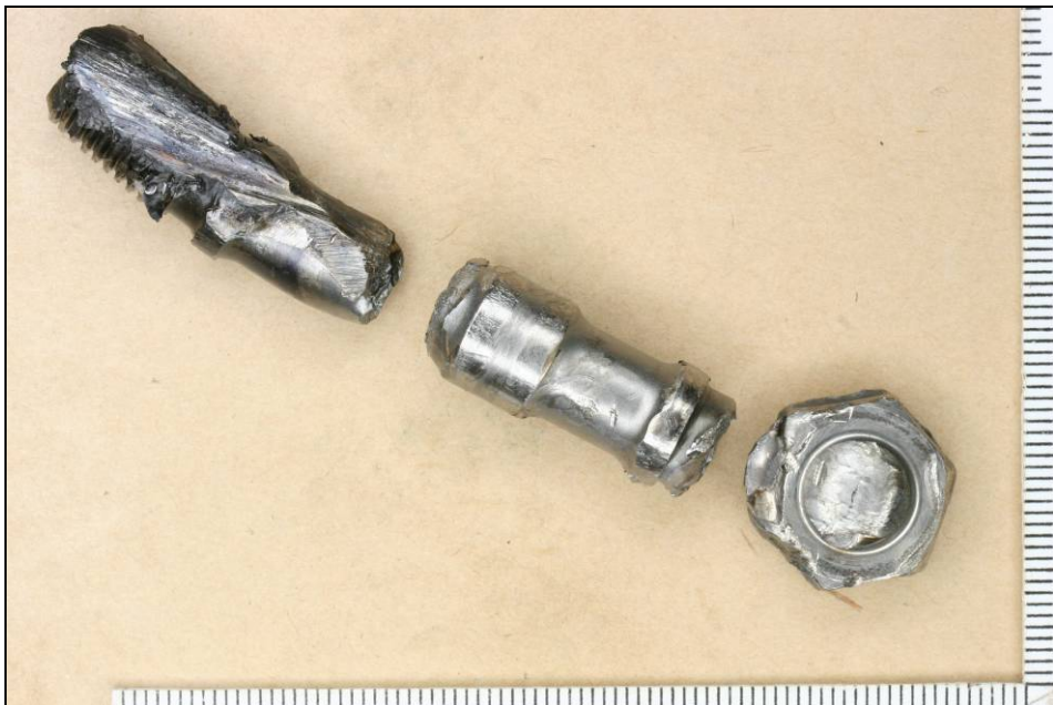
Figure 7: Number-5 connecting rod bolt 'B'
