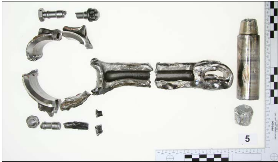
Figure 6: Number-5 cylinder connecting rod bolt and nut assembly
