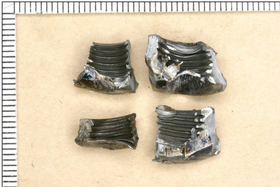
Figure 7: Fragments of nut from number-5 connecting rod bolt 'B'
