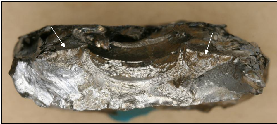
Figure 3: Fragment of the number-5 connecting rod boss, showing evidence of fatigue crack initiation and growth (arrowed areas)
