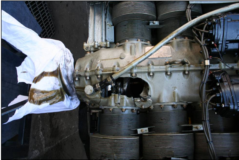
Figure 2: Damage exposed following removal of the number-6 cylinder
