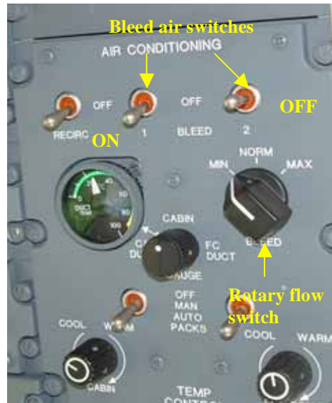
Figure 1: Overhead air conditioning panel
