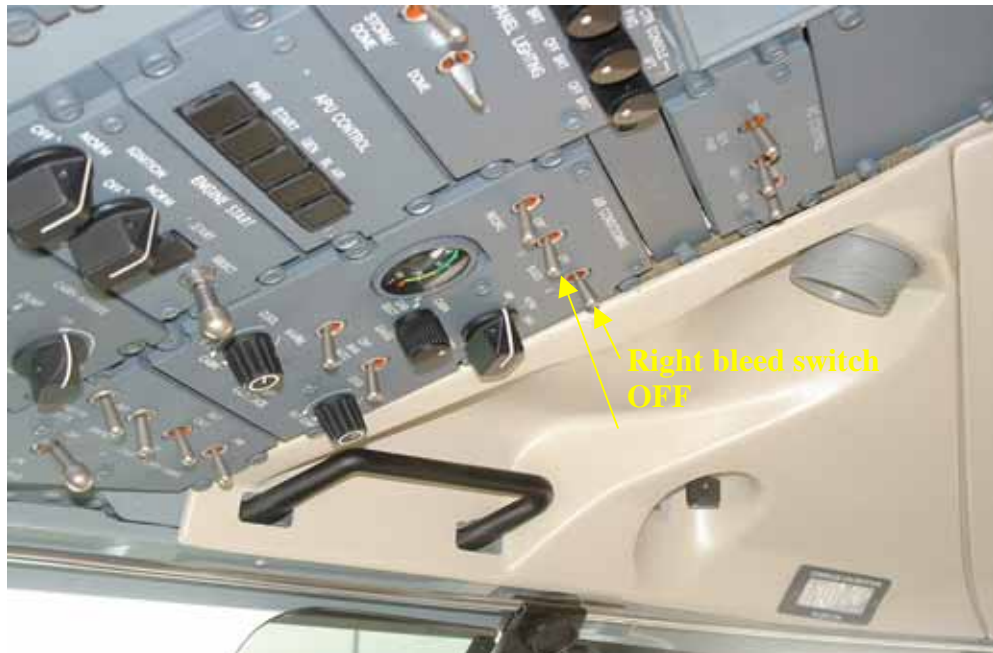
Figure 2: Daytime view of the right overhead panel from the captain's control station
