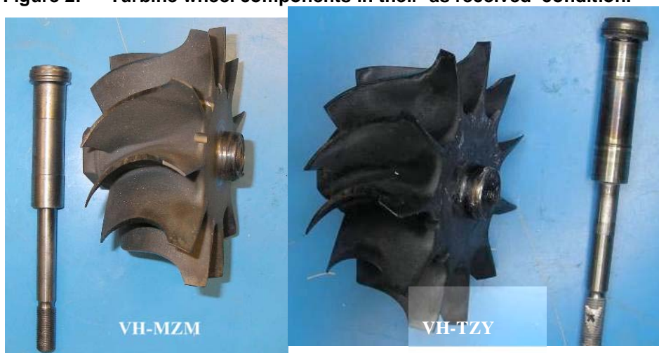
Figure 2: Turbine wheel components in their 'as received' condition.
