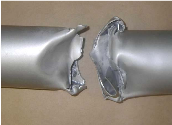
Figure 4: Fracture of the left wingspar of 32-4456.
