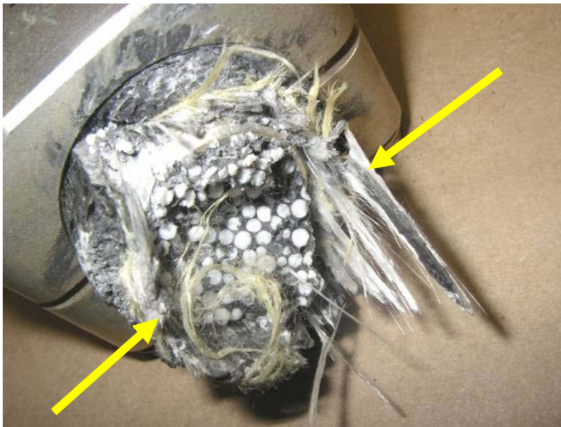
Figure 12: Fracture surface of blade C. Note fibre pull out was more pronounced on one side of the fracture surface (arrowed).
