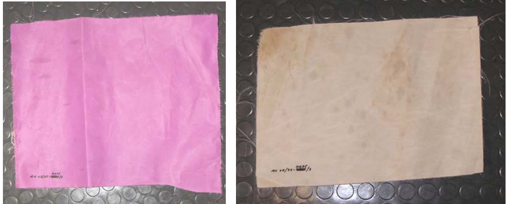
Figure 13: Purple and off-white fabric sample taken from the microlight canopy.
