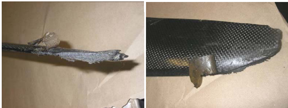
Figure 10: Leading edge damage to blade A.
