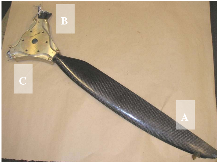
Figure 9: Fractured propeller from 32-4388.
