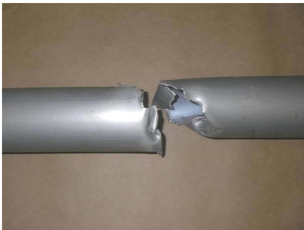
Figure 5: Fractured right wing spar of 32-4388. Note buckling and tearing features of the fracture and the 'slant' of the fracture.
