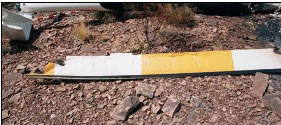
Figure 4: Compression wrinkling on main rotor blade upper surface
