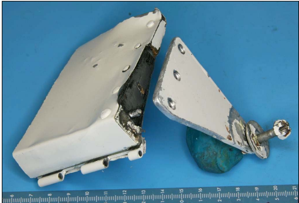
Figure 3. Detail of the control horn separation from the servo tab outer end
