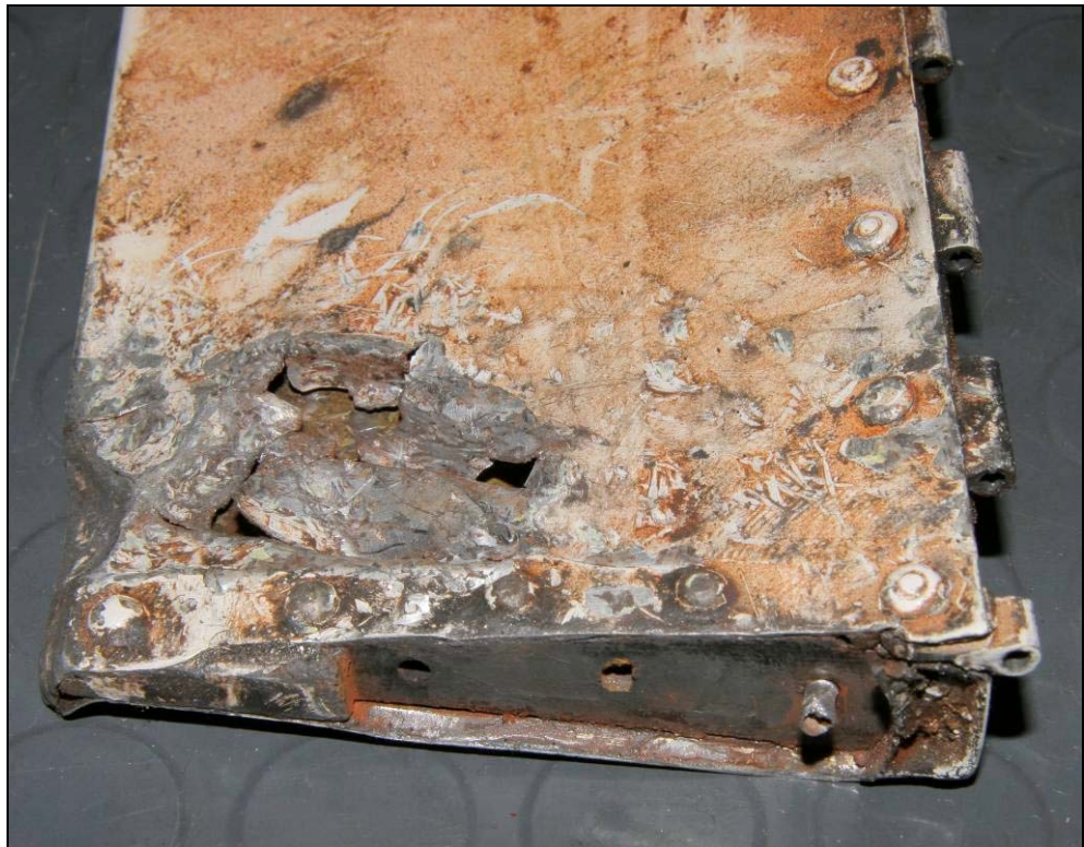
Figure 4. Damage to the upper surface of the servo tab resulting from repeated impact against the separated control horn
