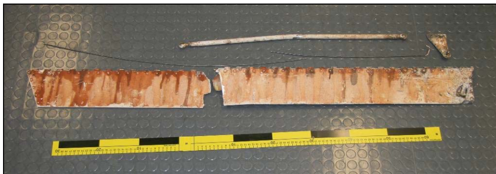
Figure 2. Servo tab removed from the VH-OTV right elevator after the event
