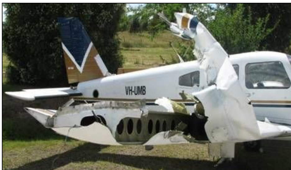
Figure 2: VH-UMB showing significant damage to right wing leading edge
