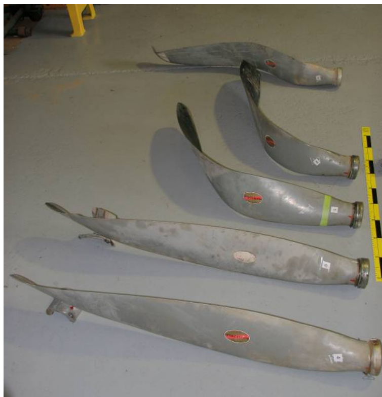
Figure 8: Propeller blade bending, reconstructed as a set
