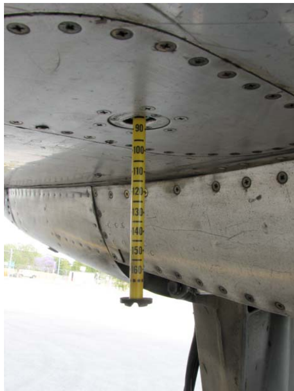
Figure 3: Magna stick in lowered position indicating 85 US gallons
