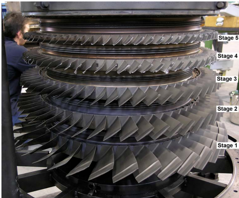
Figure 2: Photograph of the HPC rotor showing damage to the stage-four and -five rotor blades. See also Figure 3.
