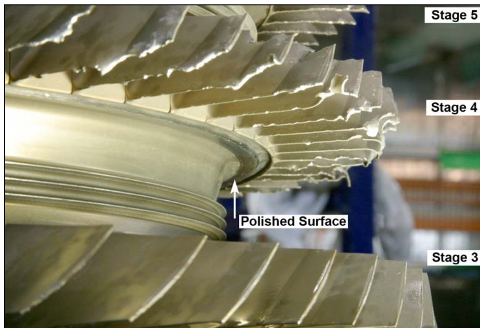
Figure 3: Close-up image of impact damage to stage-four and -five rotor blades. The forward shoulder of the dovetail slot (arrowed) shows polishing damage to the surfaces.
