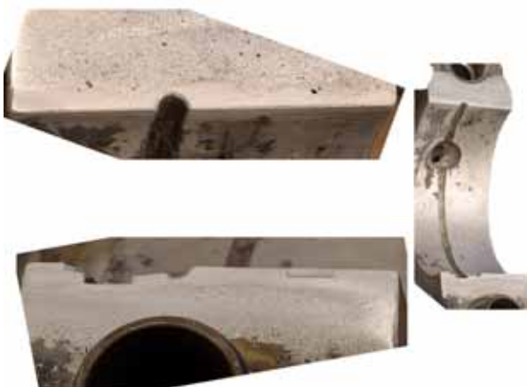
Figure 11: One half of the No.4 main bearing housing, etched to reveal the extent of weld repair
