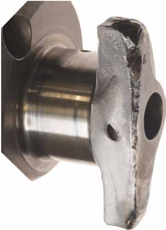
Figure 7: Crankshaft web fracture, No.3 main bearing journal/No.3 connecting rod journal
