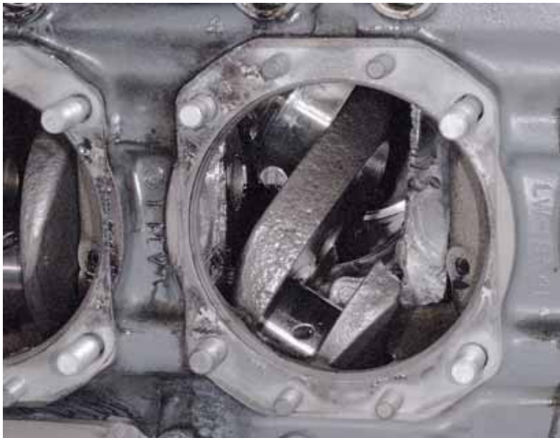
Figure 1: The fractured section of the crankshaft in the position found during initial engine examination
