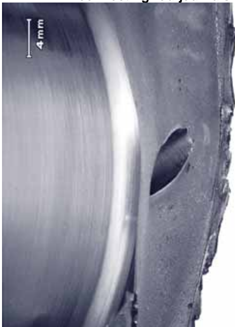
Figure 8: Detailed view of the No.3 main bearing journal fillet at the site of fatigue crack initiation in the web between the No.3 main and No.3 connecting rod journals
