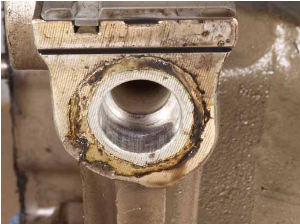
Figure 10: An example of the nature of material placed between the parting faces of each main bearing housing
