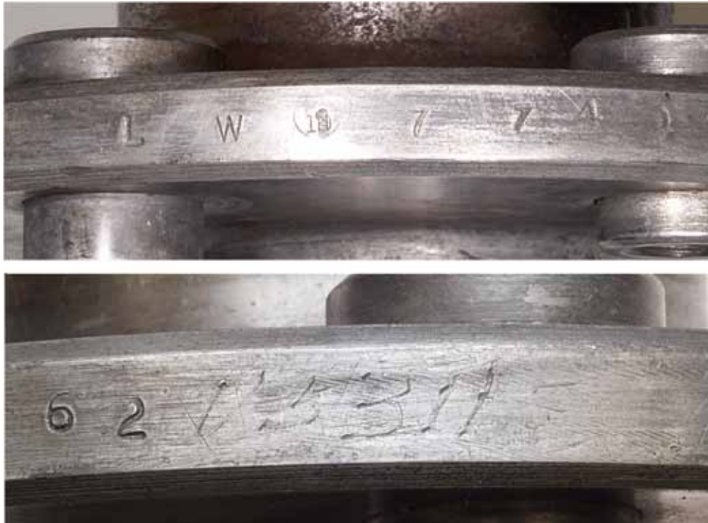
Figure 9: Crankshaft part and serial number markings on the propeller flange
