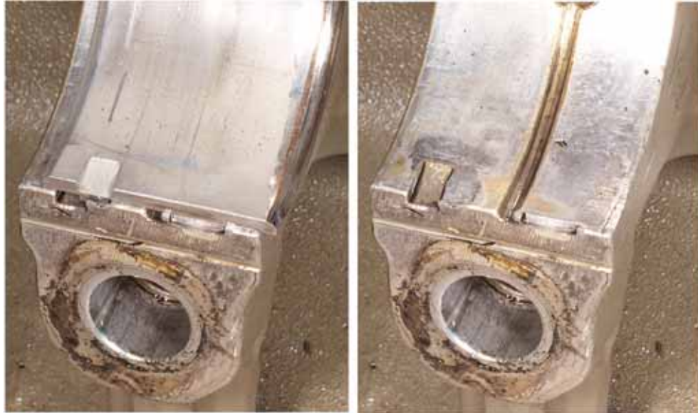
Figure 6: The extent of No.4 main bearing insert displacement
