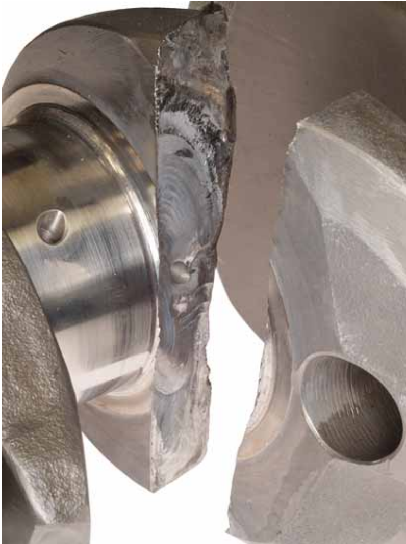
Figure 3: Crankshaft Web Fracture, No.4 main/No.4 connecting rod
