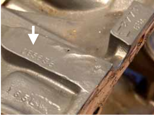
Figure 12: Weld repair crankcase marking, CG5638
