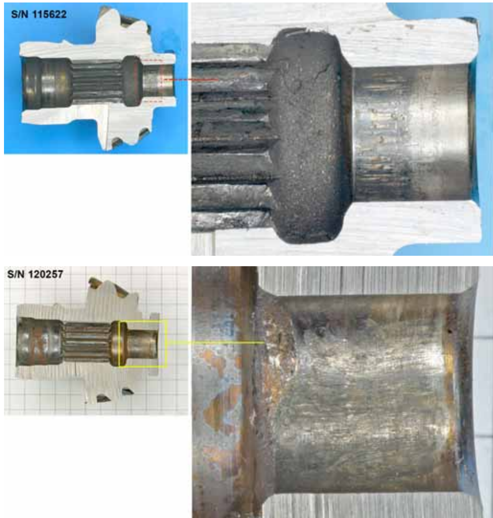
Figure 11: Close-up of the internal seating diameter from the spiral bevel gear of both engines (S/N 115622 and 120257). Axial aligned scores can be seen.
