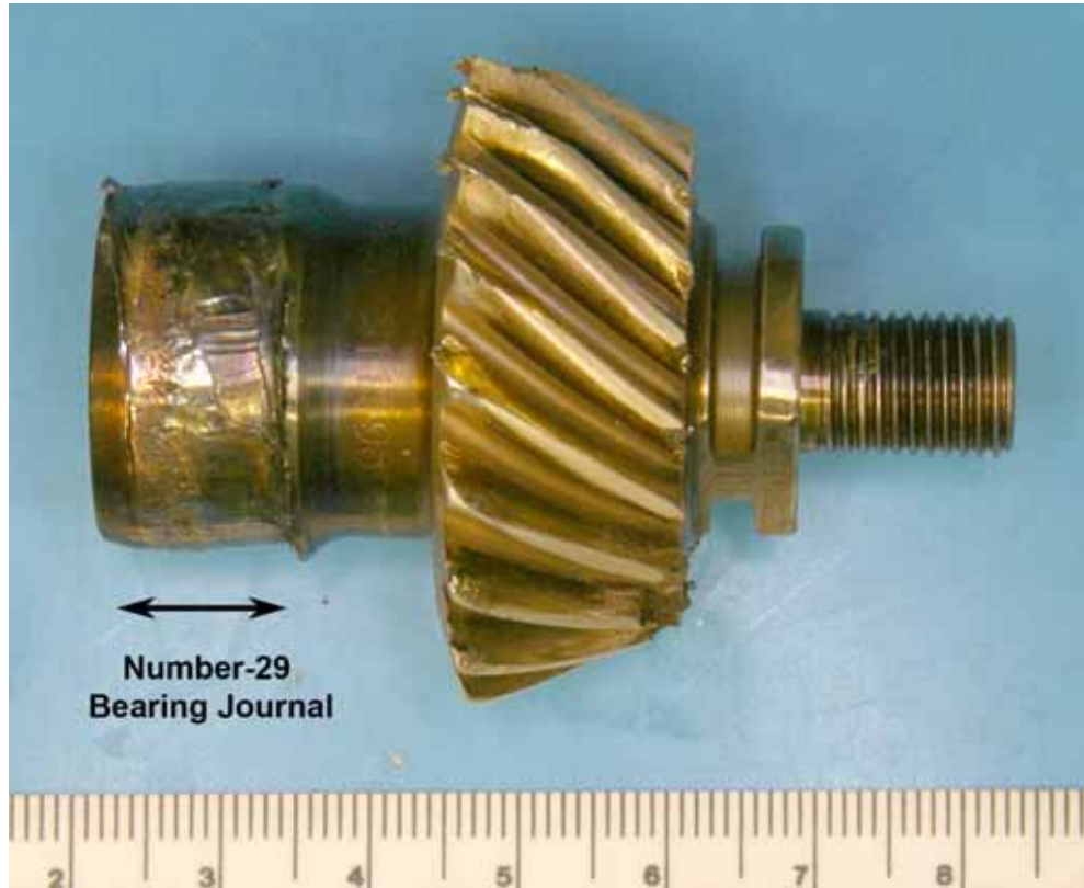
Figure 10: Photograph of the spiral bevel gear (P/N 3111969-01) from engine S/N 115622 (VH-XUD). Severe damage to the journal surface (labelled) and gear teeth had occurred. The threaded stub of the tower shaft can be seen protruding from the forward face of the gear.
