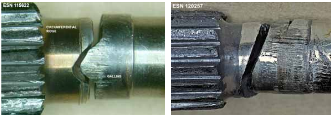
Figure 5: Close-up of fracture A-A showing the identical nature of the damage to the seating diameters of tower shafts from engine S/N 115622 (VH-XUD) and S/N 120257 (V/H TQW).
