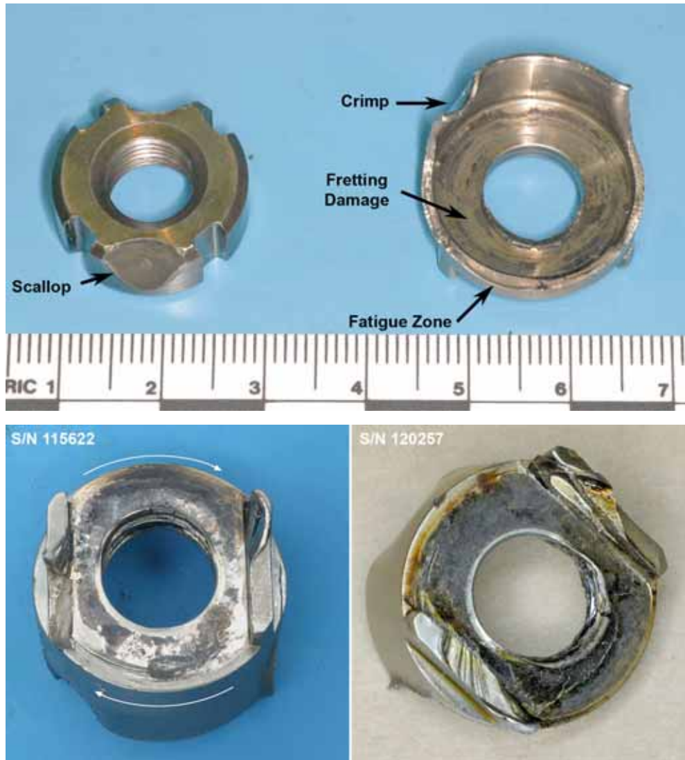
Figure 14: Top view showing the lock nut and damaged cup washer from engine S/N 115622. Identical features were observed on engine S/N 120257. Underside damage shown in lower view.
