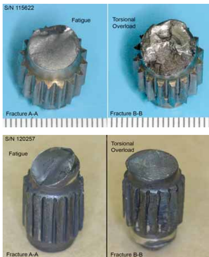
Figure 6: Opposing views of the fractured mid-shaft spline gear from engine S/N 115622 (VH-XUD) and engine S/N 120257 (VH-TQW).
