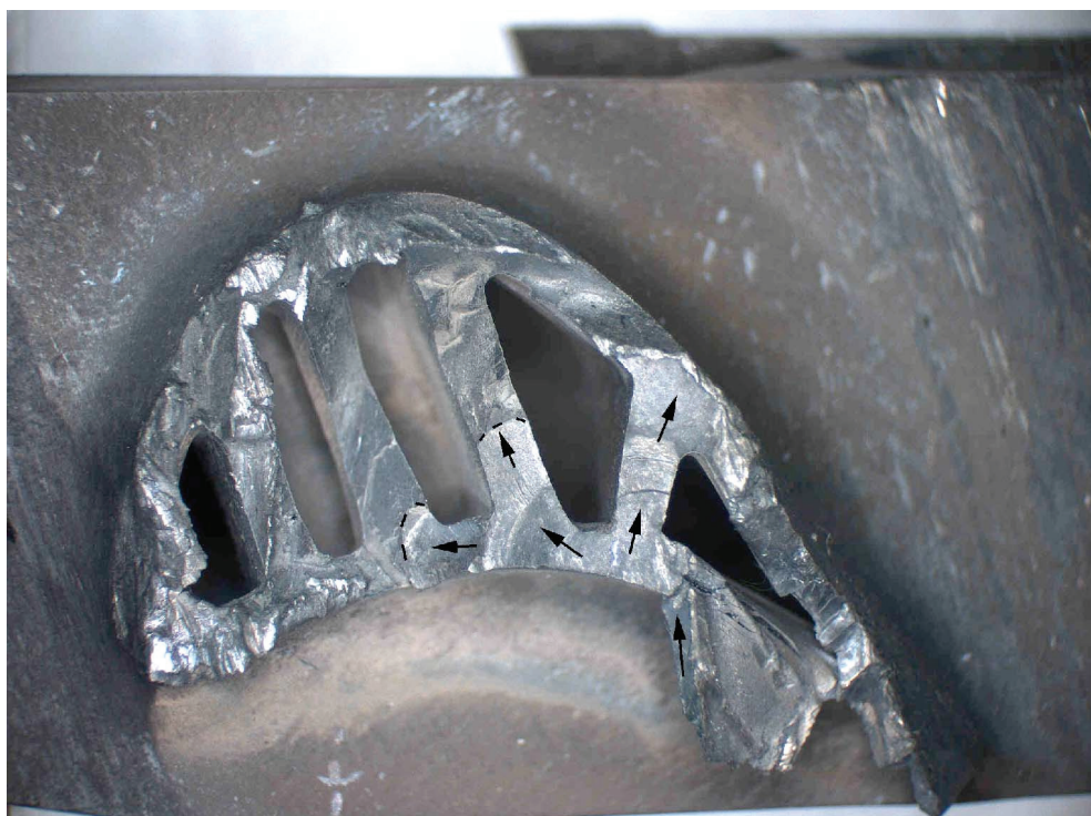
Figure 5: Fractured HPT1 blade with annotations showing the growth of fatigue cracking.
